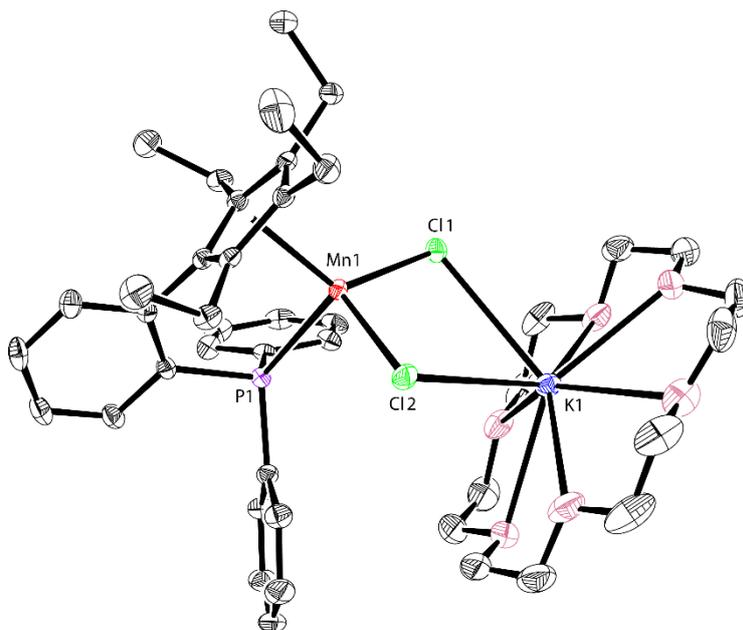
**Figure S9** ORTEP drawing of **2**. Thermal ellipsoids are shown at the 30% probability level. Hydrogen atoms are omitted for clarity.
