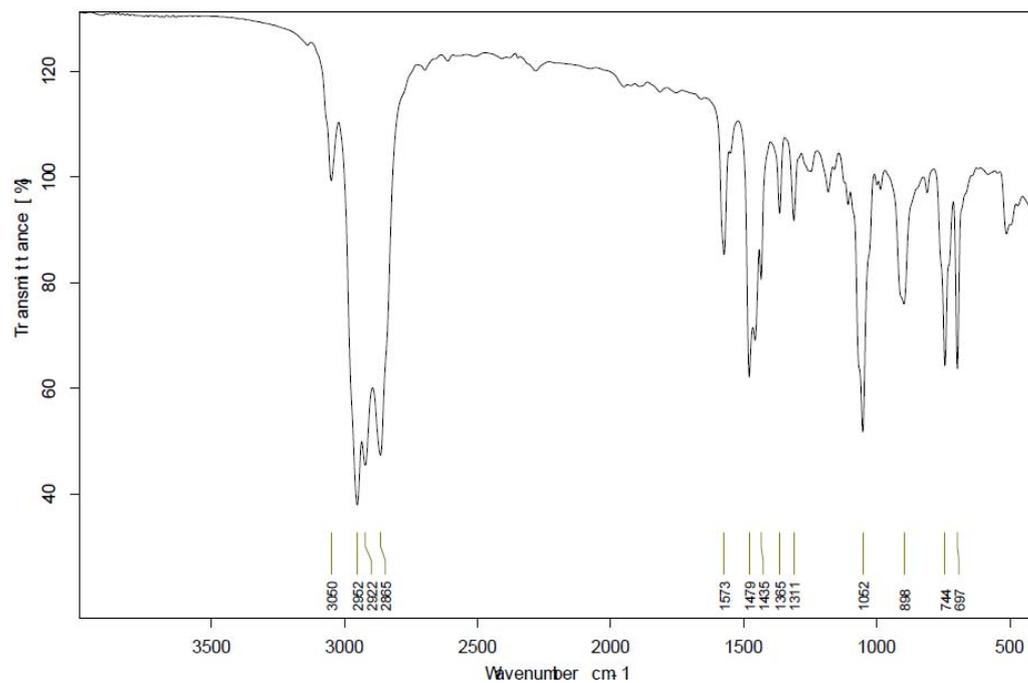
**Figure S4** IR spectra of **3** at room temperature
