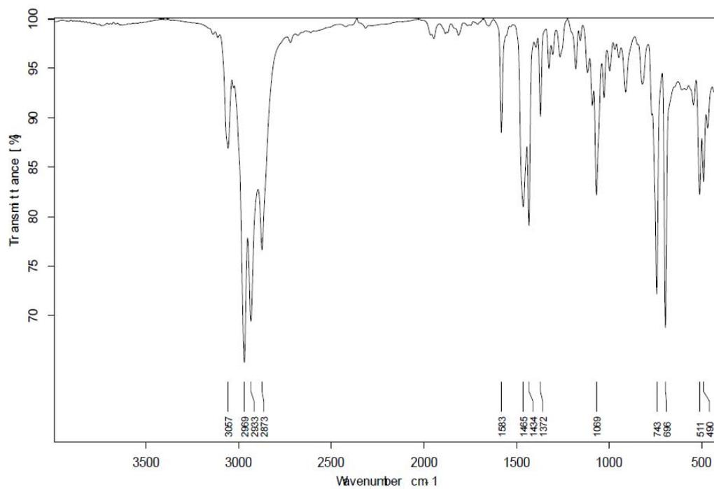
**Figure S1** IR spectra of **1a** at room temperature
