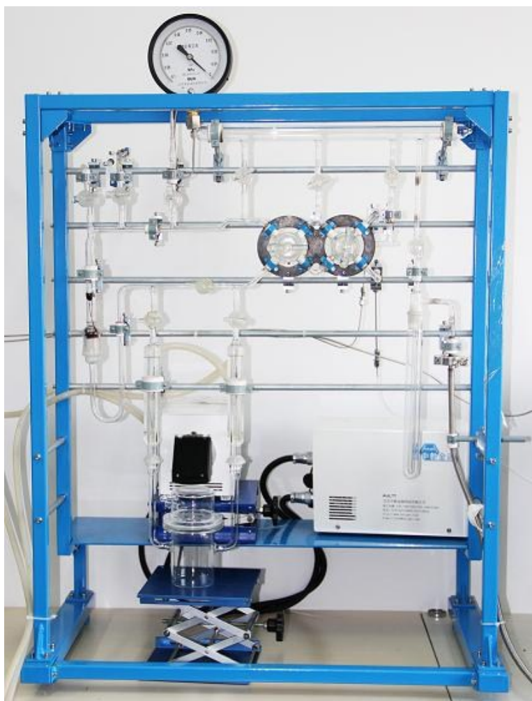
Fig. S1. The CEL-SPH2N system for photocatalytic performance tests
