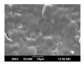
Fig.S1  $\label{eq:microstructure} \mbox{Microstructure of } \mbox{Nd}_{10}\mbox{Mo}_2\mbox{O}_{21} \mbox{ (T syn} = 1600\mbox{ }^{o}\mbox{C}).$
