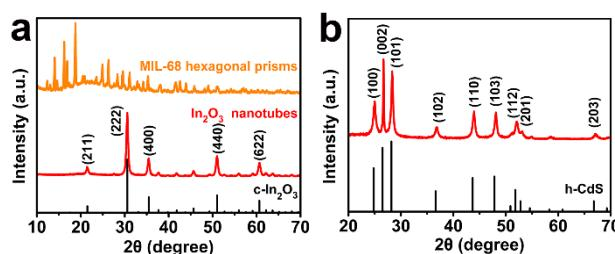
**Figure S1.** XRD patterns of (a) MIL-68 hexagonal prisms and In<sub>2</sub>O<sub>3</sub> hierarchical nanotubes, and (b) CdS nanoparticle aggregates.
