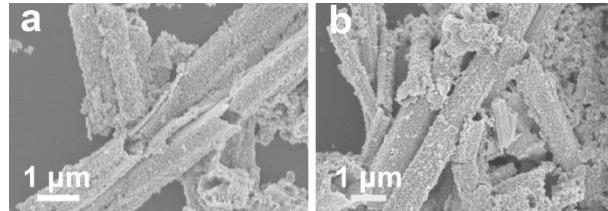
**Figure S16.** SEM images of CdS/In<sub>2</sub>O<sub>3</sub>-2 (a) before and (b) after the photocatalytic cyclic test.
