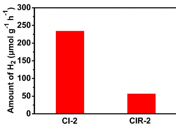
**Figure S14.** Photocatalytic activities of CdS/In<sub>2</sub>O<sub>3</sub>-2 (CI-2) and CdS/In<sub>2</sub>O<sub>3</sub> nanorods (CIR-2) towards visible-light hydrogen production from water.
