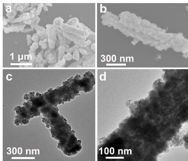
**Figure S13.** (a, b) SEM and (c, d) TEM images of CdS/In<sub>2</sub>O<sub>3</sub> nanorods.
