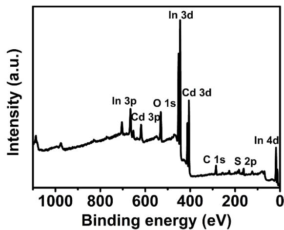
**Figure S8.** XPS survey-scan spectrum of CdS/In<sub>2</sub>O<sub>3</sub>-2.
