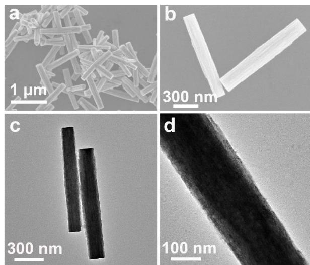
**Figure S11.** (a, b) SEM and (c, d) TEM images of  $\text{In}_2\text{O}_3$  nanorods.
