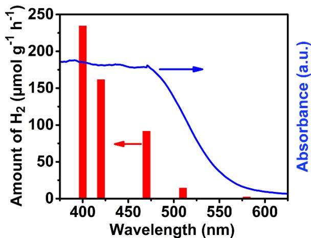
**Figure S10.** Wavelength-dependent hydrogen generation activity of CdS/In<sub>2</sub>O<sub>3</sub>-2.
