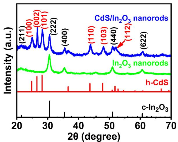
**Figure S12.** XRD patterns of the as-prepared  $\text{In}_2\text{O}_3$  nanorods and  $\text{CdS}/\text{In}_2\text{O}_3$  nanorods.
