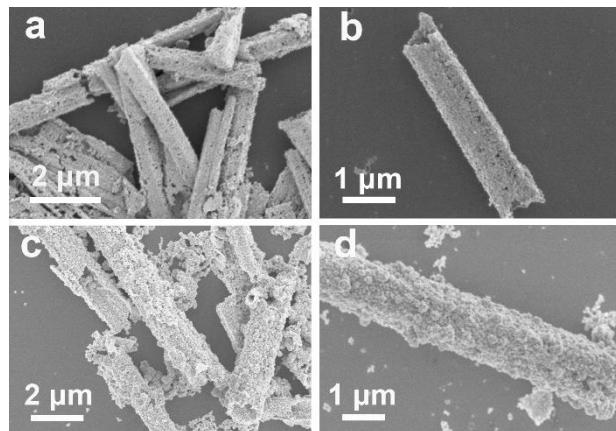
**Figure S4.** SEM images of (a, b) CdS/In<sub>2</sub>O<sub>3</sub>-1 and (c, d) CdS/In<sub>2</sub>O<sub>3</sub>-3.
