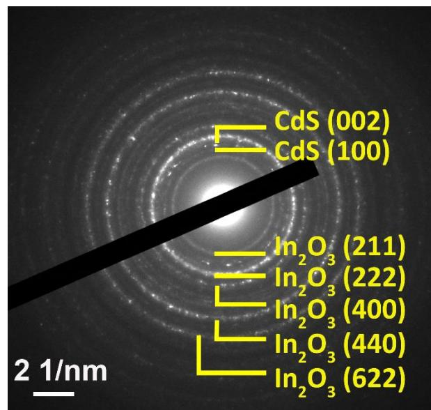
**Figure S7.** SAED pattern of CdS/In<sub>2</sub>O<sub>3</sub>-2.
