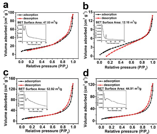
**Figure S15.** Nitrogen adsorption-desorption isotherms of (a) In<sub>2</sub>O<sub>3</sub> nanotubes, (b) CdS nanoparticles, (c) CdS/In<sub>2</sub>O<sub>3</sub>-1 and (d) CdS/In<sub>2</sub>O<sub>3</sub>-3. Insets in (a-d) are the pore size distributions of corresponding samples.
