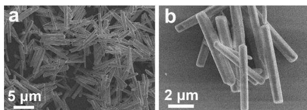
**Figure S2.** (a, b) SEM images of MIL-68 hexagonal prisms.
