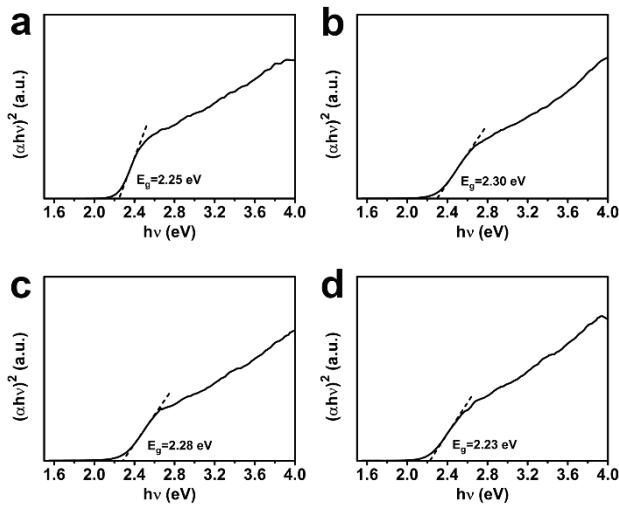
**Figure S9.** Tauc plots of (a) CdS nanoparticles, (b) CdS/In<sub>2</sub>O<sub>3</sub>-1, (c) CdS/In<sub>2</sub>O<sub>3</sub>-2 and (d) CdS/In<sub>2</sub>O<sub>3</sub>-3.
