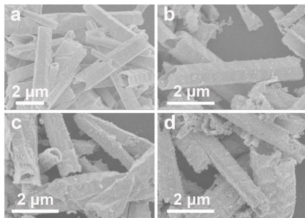
**Figure S5.** SEM images of CdS/In<sub>2</sub>O<sub>3</sub>-2 at (a) 10 min, (b) 30 min, (c) 60 min and (d) 120 min in the growth process of CdS.
