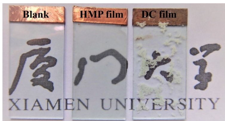
Figure S4. Optical pictures of large-scale uniform HMP films prepared on ITO-glass (middle), with blank glass (left) and the drop-casting film (right) as contrast.
