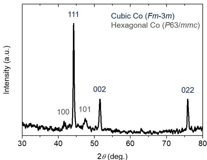
**Fig. S2** XRD pattern of the inorganic residue obtained after TGA analysis of the CoO mesoporous sample (up to 600 °C, in  $N_2$ ). All diffraction peaks could be indexed to the metallic Co with a face-centered cubic (JCPDS No. 15-0806) and hexagonal close-packed (JCPDS No. 05-0727) structure.
