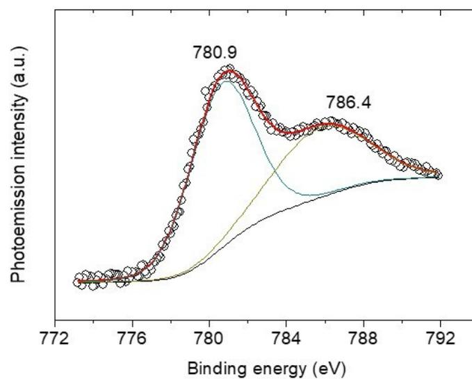
**Fig. S9** Co  $2p_{3/2}$  XPS spectrum of the  $\text{Co}_{0.98}\text{Ni}_{0.02}\text{O}$  MNAs catalyst obtained after catalysis, showing a Co  $2p_{3/2}$  peak at 780.9 eV associated with a shake-up satellite peak at 786.4 eV.
