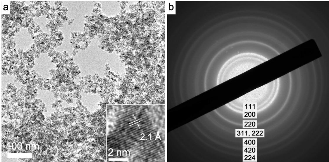
**Fig. S3** (a) Typical TEM images and (b) SAED pattern of CoO MNAs.
