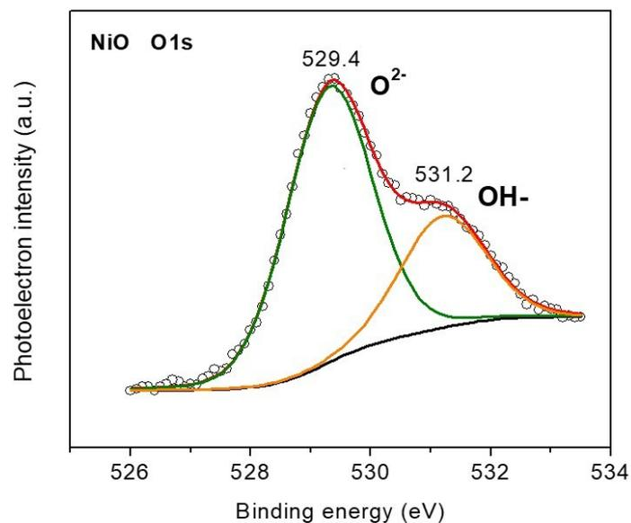
**Fig. S5** O 1s XPS spectrum of the polycrystalline NiO material.
