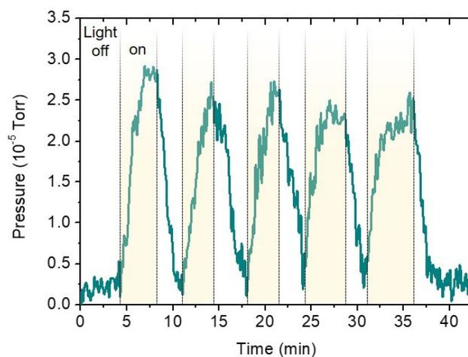
**Fig. S10**  $\text{O}_2$  evolution transient with light on/off for  $\text{Co}_{0.98}\text{Ni}_{0.02}\text{O}$  MNAs catalyst under  $\lambda > 360$  nm light irradiation.
