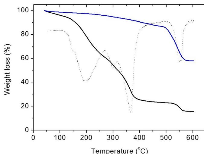
**Fig. S1** TGA profiles of (a) as-prepared containing surfactant (black line) and (b) mesoporous CoOMNAs recorded under  $N_2$  flow ( $\sim 200 \text{ mL min}^{-1}$ ). The differential thermogravimetric (DTG) curve (dotted line) for as-prepared material is also given.
