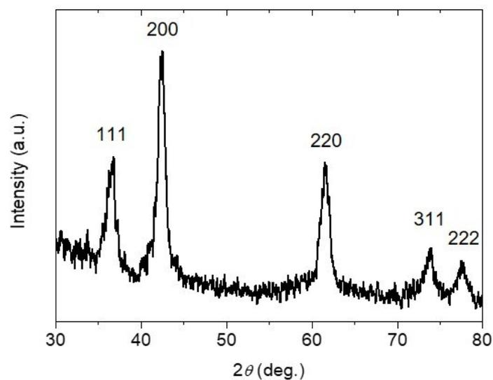
**Fig. S7** Powder XRD pattern of the reused  $\text{Co}_{0.98}\text{Ni}_{0.02}\text{O}$  MNAs catalyst. All the diffraction peaks in the XRD pattern can be assigned to the cubic phase of  $\text{CoO}$  (JCPDS No. 43-1004).
