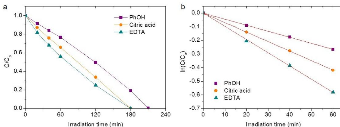
**Fig. S12** (a) Photocatalytic reduction of aqueous Cr(VI) and (b) kinetic profiles over Co<sub>0.98</sub>Ni<sub>0.02</sub>O MNAs catalyst in the presence 1 equiv. of phenol, citric acid or EDTA under  $\lambda > 360$  nm light irradiation. Reaction conditions: 0.3 g L<sup>-1</sup> catalyst, 50 mg L<sup>-1</sup> Cr(VI) solution, pH = 2, 20 °C. In panel (b), the red lines are fit to the data.
