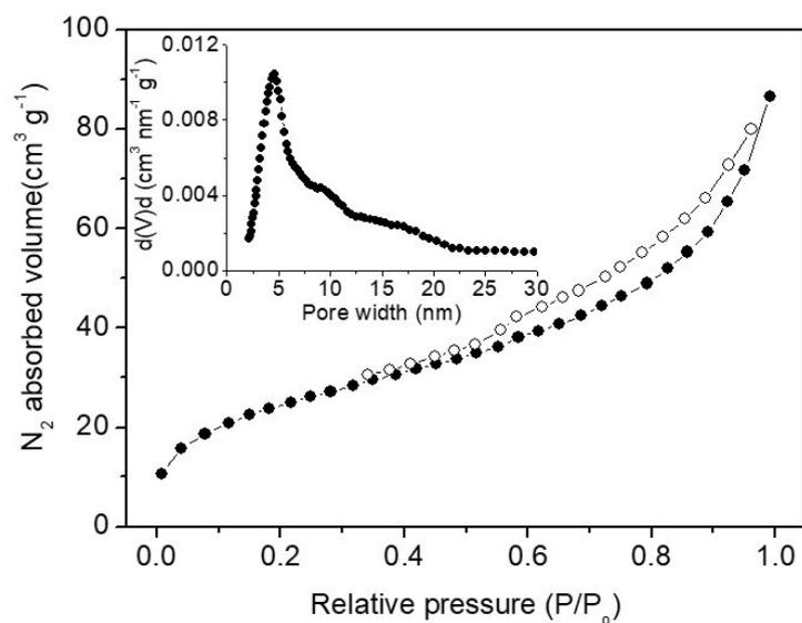
**Fig. S8**  $\text{N}_2$  adsorption-desorption isotherms at  $-196\text{ }^\circ\text{C}$  (Inset: the corresponding NLDFT pore size distribution, indicating an average pore size of  $\sim 4.6\text{ nm}$ ) of the  $\text{Co}_{0.98}\text{Ni}_{0.02}\text{O}$  MNAs catalyst retrieved after the cycling test. Analysis of the adsorption data indicate a BET surface area of  $92\text{ m}^2\text{g}^{-1}$  and a pore volume of  $0.13\text{ cm}^3\text{g}^{-1}$ .
