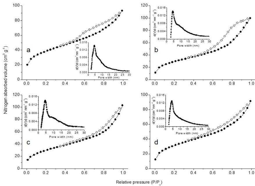
**Fig. S4**  $N_2$  adsorption (filled cycles) and desorption (open cycles) isotherms at  $-196\text{ }^\circ\text{C}$  and the corresponding NLDFT pore-size distribution (insets) for  $\text{Co}_{1-x}\text{Ni}_x\text{O}$  MNAs: (a)  $x = 0$ , (b)  $x = 0.01$ , (c)  $x = 0.02$  and (d)  $x = 0.05$ . All the materials showed type-IV adsorption-desorption isotherms with a  $H_3$  type hysteresis loop, which is characteristic of mesoporous solids with slit-like pores.
