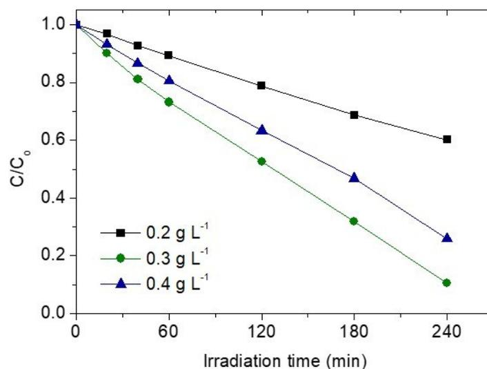
**Fig. S6** Concentration dependent photocatalytic Cr(VI) reduction activity of Co<sub>0.96</sub>Ni<sub>0.02</sub>O MNAs. Reaction conditions: 0.2–0.4 g L<sup>-1</sup> of catalyst, 50 mg L<sup>-1</sup> Cr(VI) aqueous solution, pH = 2, UV-visible light ( $\lambda > 360$  nm) irradiation, 20 °C.
