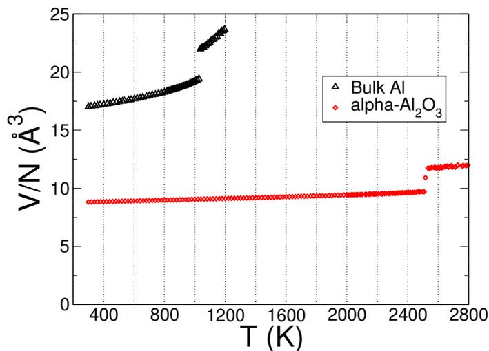
Fig. 1 Volume per atom versus temperature curves, for Al and  $\alpha\text{-Al}_2\text{O}_3$  bulks.
