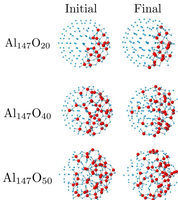
**Fig. 3** Clusters of  $\text{Al}_{147}\text{O}_{20}$ ,  $\text{Al}_{147}\text{O}_{40}$  and  $\text{Al}_{147}\text{O}_{50}$  after a energy minimization. Initial configurations are considered from MD simulations. Light blue and red atoms correspond to O and Al atoms respectively.
