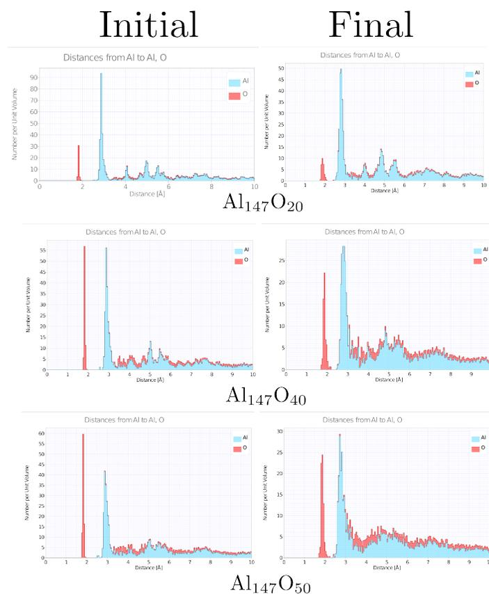
**Fig. 4** Bonds length for  $\text{Al}_{147}\text{O}_{20}$ ,  $\text{Al}_{147}\text{O}_{40}$  and  $\text{Al}_{147}\text{O}_{50}$  after a energy minimization. Initial configurations its taken after a previos MD simulations.
