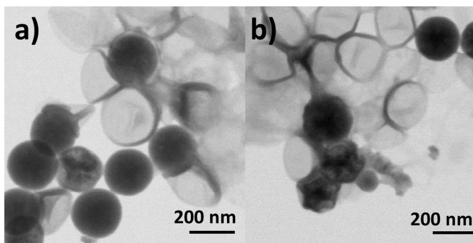
**Figure S18** Details of STEM images of a) **Im-MSP-10%** and b) **Im-MSPs-25%** at 0.1 mg/mL in AcOH/AcONa buffer solution at pH 5.2 at a) and b) 3h; c) 1d; d) 5d.
