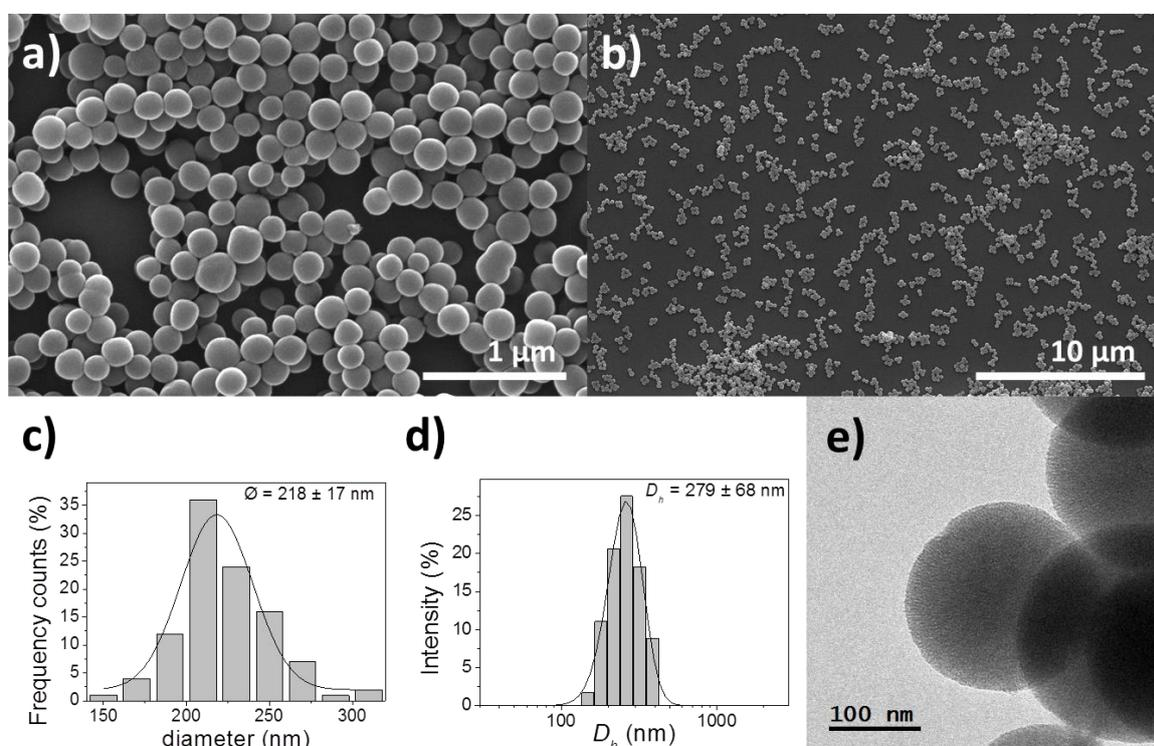
**Figure S1** a) and b) Additional SEM pictures of **MSPs**, c) size distribution from SEM micrographs, counts on 100 particles, the mean diameter was extrapolated from the Gaussian distribution, d) DLS intensity distribution of **MSPs** dispersed in EtOH, e) additional TEM image of **MSPs**.
