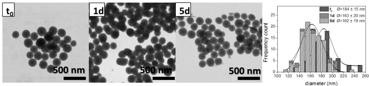
**Figure S19** STEM images of MSPs in acetate buffer (pH 5.2) at r.t. at  $t_0$  and after 1 and 5d. On the right the size distributions of the imaged particles are reported.
