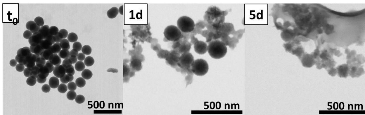
**Figure S20** STEM images on MSPs in PBS (pH 7.4) at r.t. at  $t_0$  and after 1 and 5d.
