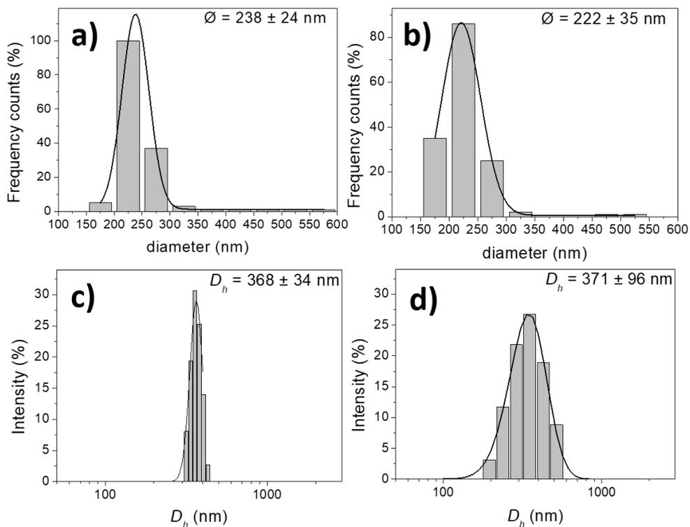
**Figure S6** Size distribution from SEM micrographs of a) **Im-MSPs-10%** and b) **Im-MSPs-25%** after purification. The distribution was calculated on 150 particles. The mean diameter values were extrapolated from the Gaussian distribution. DLS intensity distribution of c) **Im-MSPs-10%** and d) **Im-MSPs-25%**. The slight larger values determine from DLS can be attributed to the presence of aggregates, given the hydrophobic nature of the organic functionalization.
