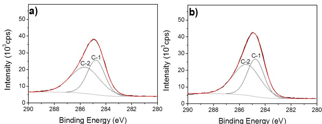
**Figure S8.** XPS high resolution scans of C(1s) level recorded on a) **Im-MSPs-10%** and b) **Im-MSPs-25%** (black lines) and calculated peak (red line). The deconvolution of the peak reveals the presence of two components (C-1 and C-2). The C-1 component (284.8 eV) can be attributed to C-C, C-H and C-Si while the second component C-2 (285.5 eV) to C=N and aromatic C. The ratio between the two components is 44:56 for both **Im-MSPs-10%** and **Im-MSPs-25%**.
