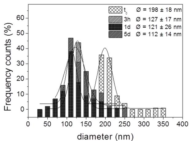
**Figure S17** Size distributions calculated from STEM micrographs of **Im-MSPs-25%** in AcOH/AcONa buffer solution (pH 5.2) over time. Counts performed on 100 particles. The distributions at 3h, 1d and 5d have been calculated only on the particles that could be imaged, and they are not representative of the entire sample.
