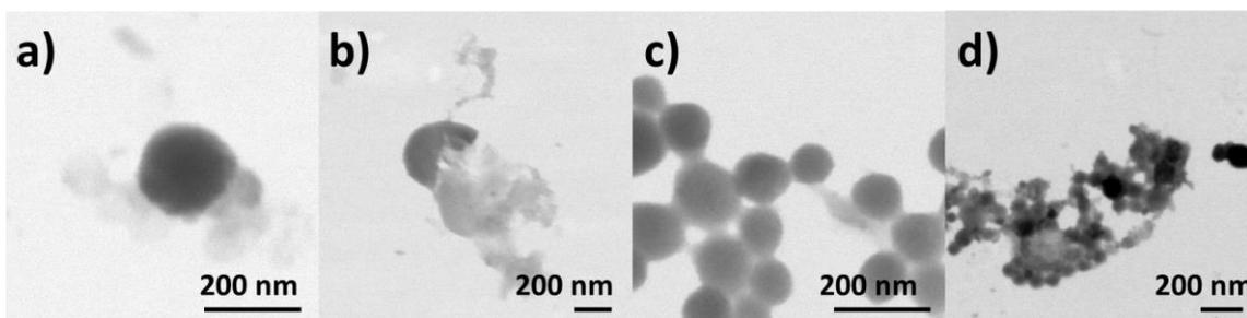
**Figure S14** Details of STEM images of **Im-MSPs-10%** 0.1 mg/mL in AcOH/AcONa buffer solution at pH 5.2 at a) and b) 3h; c) 1d; d) 5d (zoom of Figure 6a, 5d).
