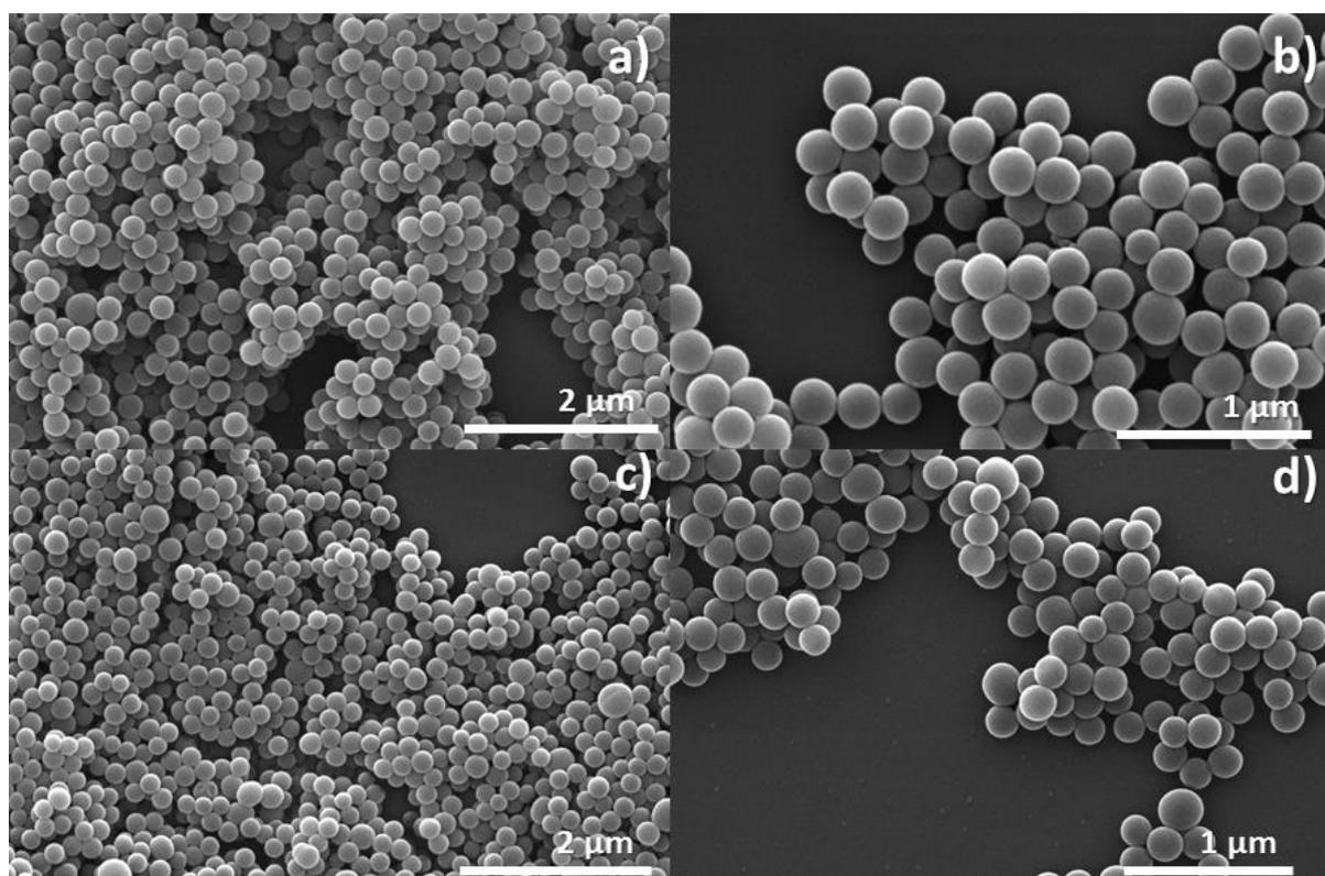
**Figure S5.** Additional SEM images of the purified a) and b) **Im-MSPs-10%**; c) and d) **Im-MSPs-25%**.
