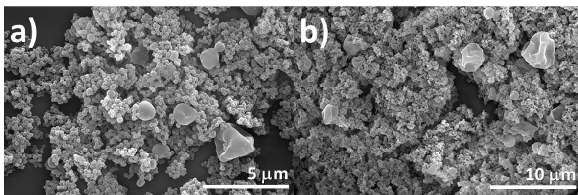
**Figure S4.** SEM images recorded on the precipitate left after the purification by means of centrifugation cycles on a) **Im-MSPs-10%** and b) **Im-MSPs-25%**.
