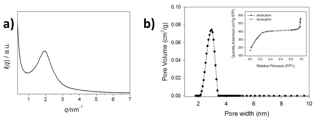
**Figure S2** a) SAXS patterns recorded on **MSPs**; b) Adsorption/desorption isotherm obtained on **MSPs**, in the inset the pore width distribution.
