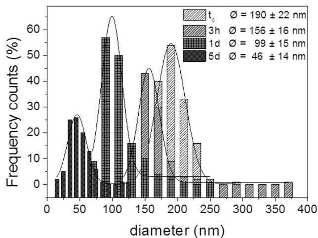
**Figure S16** Size distributions calculated from STEM micrographs of **Im-MSPs-10%** in AcOH/AcONa buffer solution (pH 5.2) over time. Counts performed on 100 particles. The distributions at 3h, 1d and 5d have been calculated on the particles that could be visualized, and they are not representative of the entire sample.
