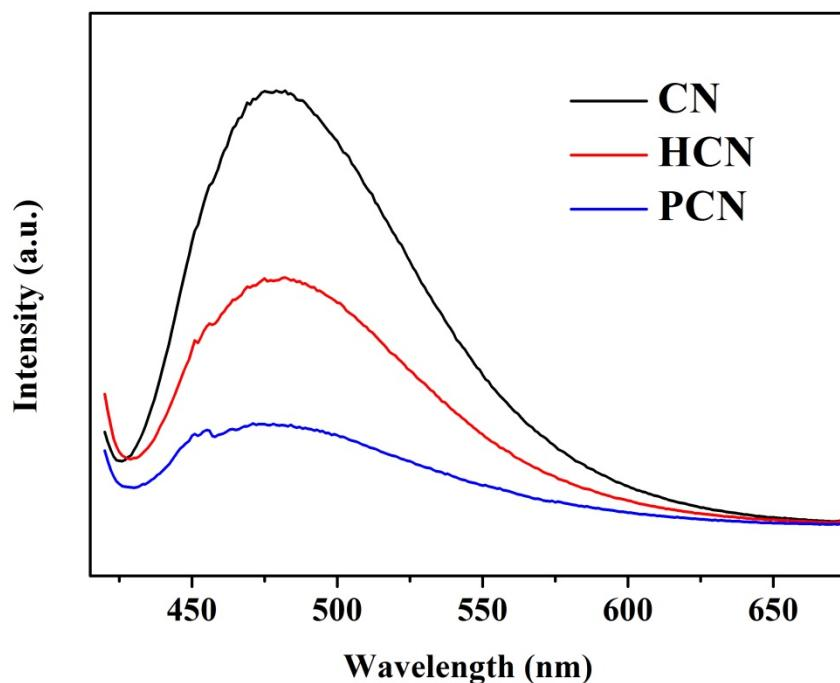
**Fig. S8.** PL spectra of CN, HCN and PCN.
