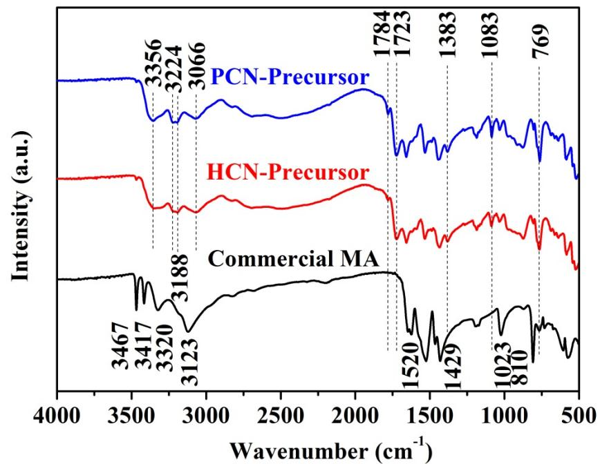
**Fig. S2.** FTIR spectra of the commercial MA, HCN-precursor and PCN-precursor.
