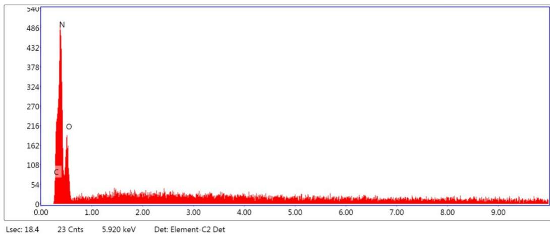
**Fig. S1.** EDS result of the *Coca-Cola*-assisted hydrothermal-reformed MA precursor.
