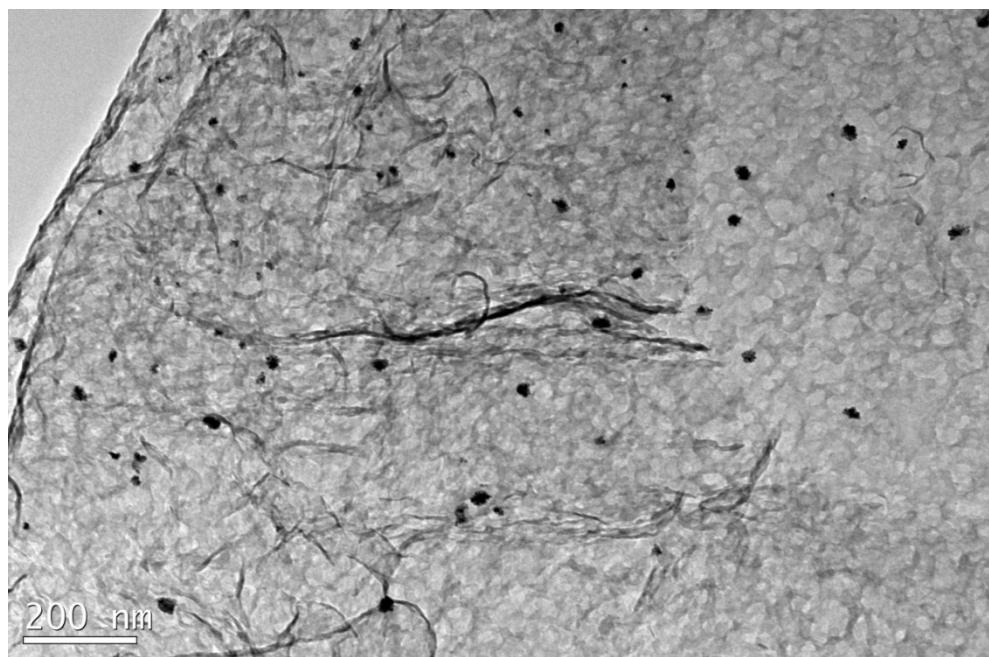
**Fig. S5.** TEM image of the PCN sample after the photocatalytic hydrogen evolution reaction after three successive cycles.
