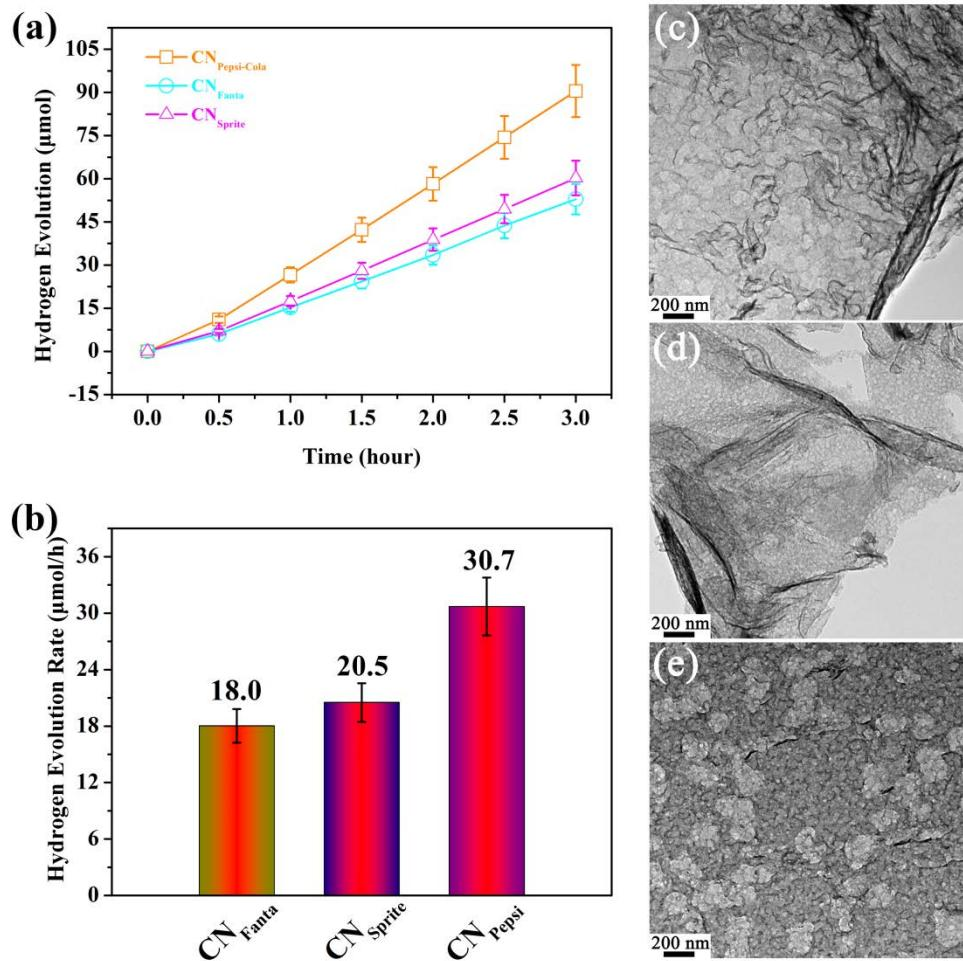
**Fig. S4.** (a) Photocatalytic H<sub>2</sub> evolution by the CN<sub>Pepsi-Cola</sub>, CN<sub>Sprite</sub> and CN<sub>Fanta</sub> photocatalysts under visible light irradiation. (b) HER of the CN<sub>Pepsi-Cola</sub>, CN<sub>Sprite</sub> and CN<sub>Fanta</sub>. (c) ~ (e) TEM images of CN<sub>Pepsi-Cola</sub>, CN<sub>Sprite</sub> and CN<sub>Fanta</sub>, respectively.
