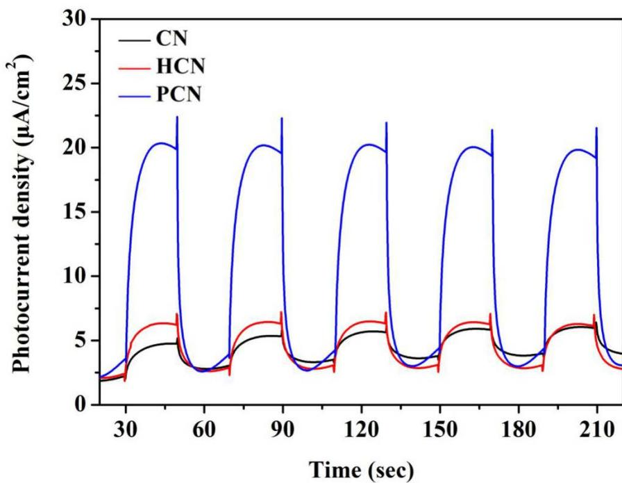
**Fig. S6.** Transient photocurrent responses of CN, HCN and PCN under visible-light irradiation.
