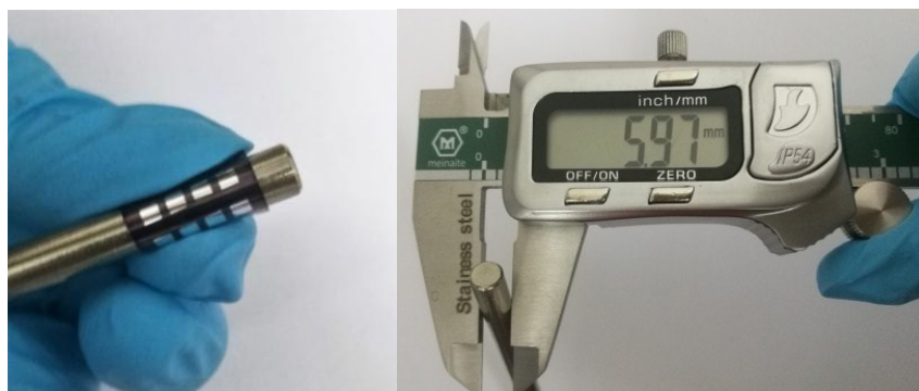
Fig. S6 The picture of bend test station and cylindrical radius
