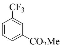
**Methyl 3-(trifluoromethyl)benzoate (3f)**<sup>1</sup>: The reaction was run on substrate (0.5 mmol), FSO<sub>2</sub>CF<sub>2</sub>CO<sub>2</sub>Me (1.25 mmol, 2.5 equiv), and CuCl<sub>2</sub> (0.05 mmol, 0.1 equiv), and the product was obtained as a colorless liquid in 86% yield by silica gel flash
