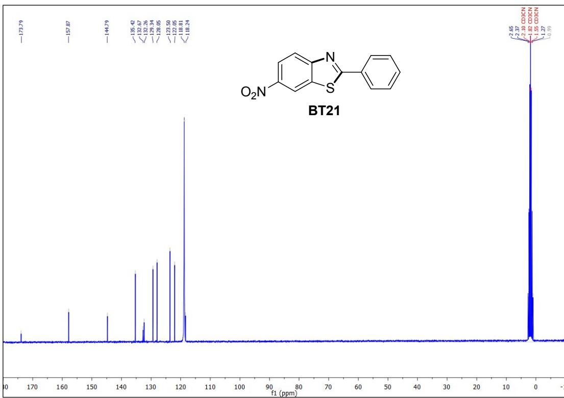
**Figure S21.**  $^1\text{H}$  (top, 300 MHz) and  $^{13}\text{C}$  (bottom, 75 MHz) NMR spectra of **BT21** in  $\text{CD}_3\text{CN}$ .
