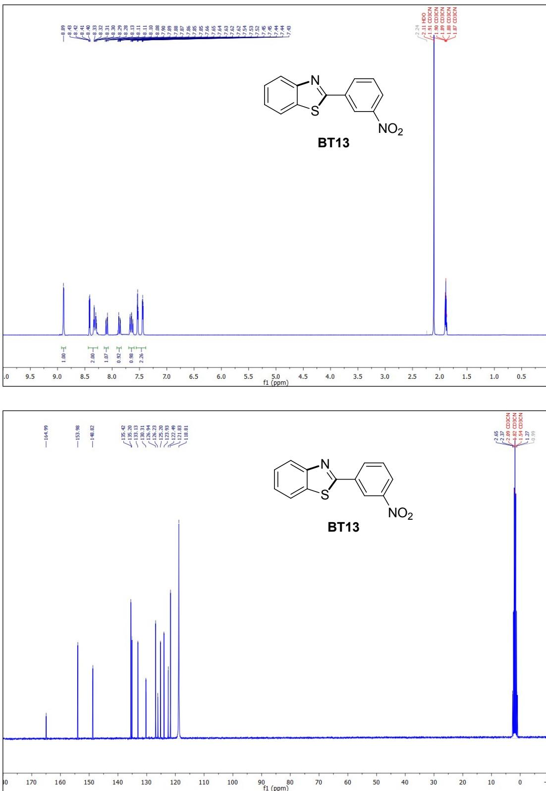
**Figure S13.**  $^1\text{H}$  (top, 300 MHz) and  $^{13}\text{C}$  (bottom, 75 MHz) NMR spectra of **BT13** in  $\text{CD}_3\text{CN}$ .
