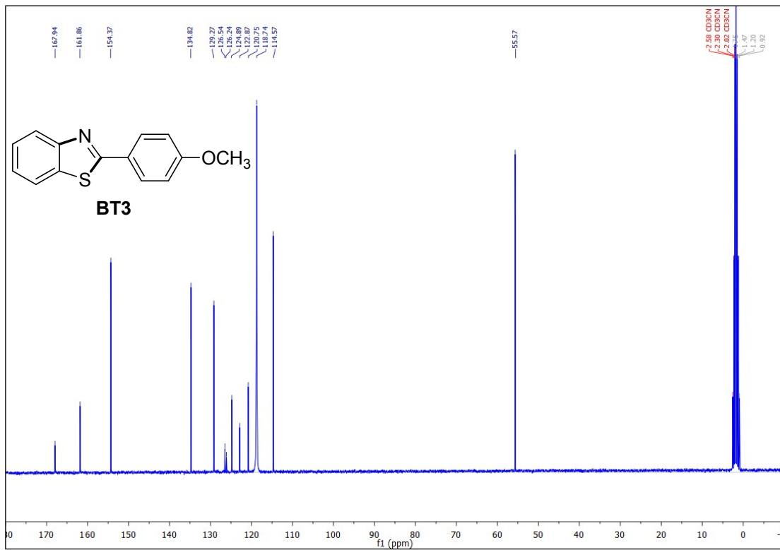
**Figure S3.**  $^1\text{H}$  (top, 300 MHz) and  $^{13}\text{C}$  (bottom, 75 MHz) NMR spectra of **BT3** in  $\text{CD}_3\text{CN}$ .
