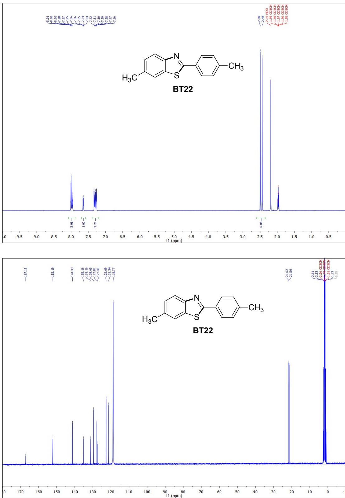
**Figure S22.**  $^1\text{H}$  (top, 300 MHz) and  $^{13}\text{C}$  (bottom, 75 MHz) NMR spectra of **BT22** in CD<sub>3</sub>CN.
