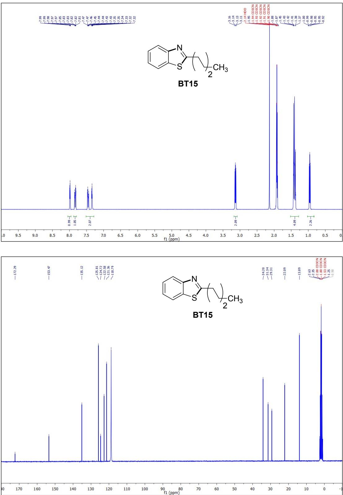
**Figure S15.**  $^1\text{H}$  (top, 300 MHz) and  $^{13}\text{C}$  (bottom, 75 MHz) NMR spectra of **BT15** in  $\text{CD}_3\text{CN}$ .
