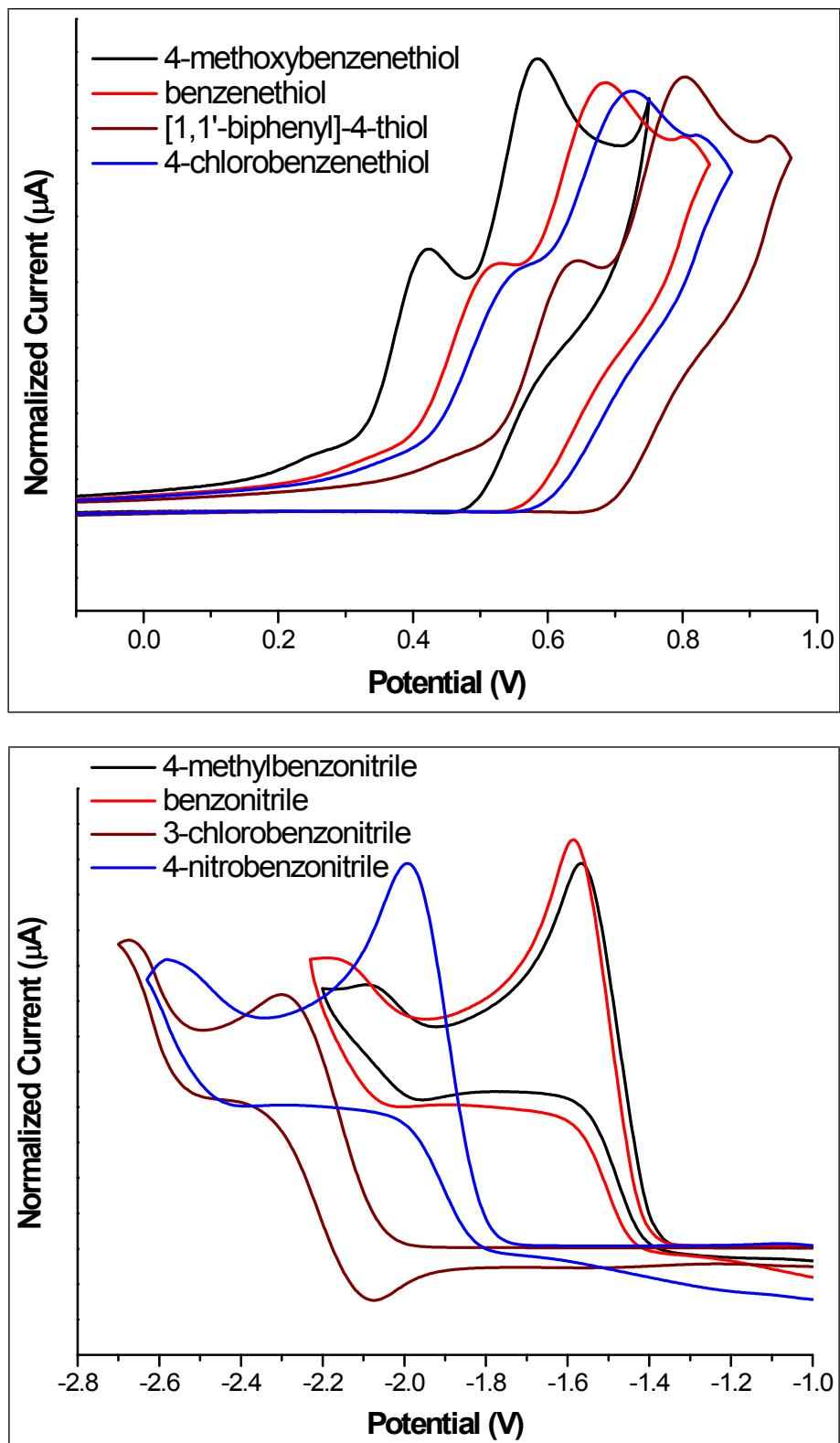
**Figure S1.** The cyclic voltammogram of aryl thiols (top) and aryl nitriles (bottom) at a scan rate of 50 mV/s.
