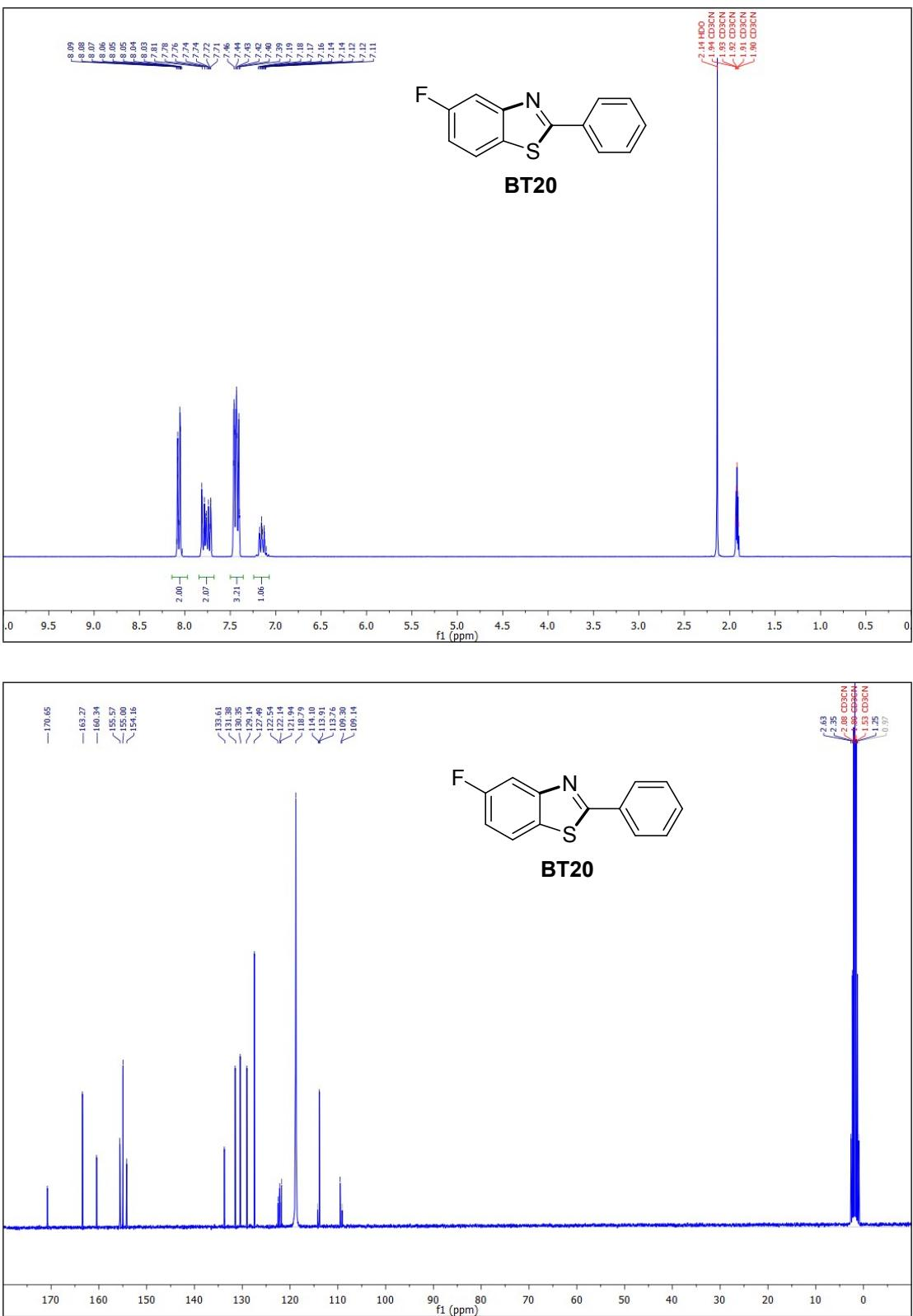
**Figure S20.**  $^1\text{H}$  (top, 300 MHz) and  $^{13}\text{C}$  (bottom, 75 MHz) NMR spectra of **BT20** in  $\text{CD}_3\text{CN}$ .
