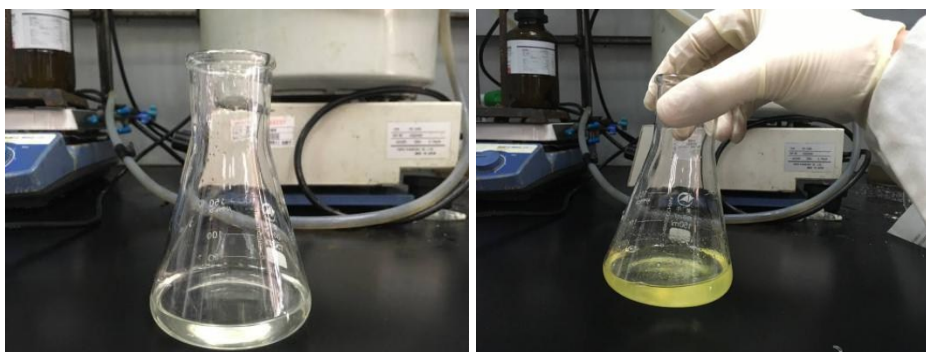
Supporting Figure 1 Left: 1,2-diphenyldisulfane and 2-(Difluoromethylsulfonyl)pyridine were dissolved in DMF; Right :slightly shook after the addition of t -BuONa ( about 5 seconds)
