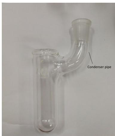
Figure S1. The structure of the undivided cell
