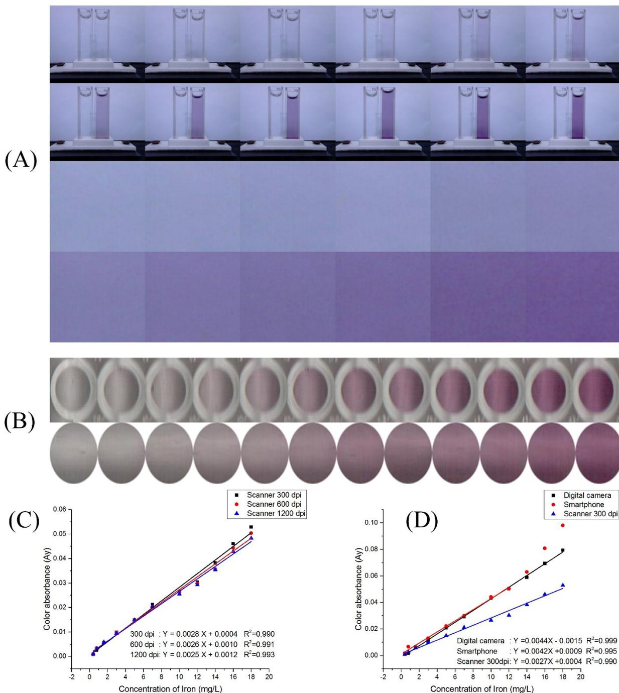
**Fig. S6.** Digital images and cropped images of Fe(III)-salicylate standard solutions (0.0-18.0 mg L<sup>-1</sup> Fe). Images captured using (A) a Sony Xperia E smartphone with a 3.15 MP camera and (B) the scanner of HP LaserJet Pro M1536dnf MF printer at 1200 dpi. Calibration graphs based on images from desktop scanner at 300, 600 and 1200 dpi (C), and from different image-capturing devices (D). The other conditions tested are those shown in **Fig. S2**.
