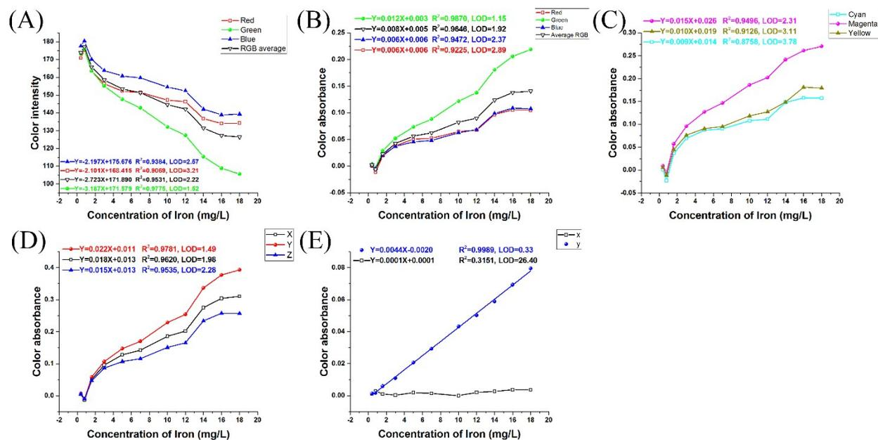
**Fig. S4.** Calibration curves of the Fe(III)-salicylate System; responses are (A) RGB intensity, (B) RGB colour absorbance, (C) CMY colour absorbance, (D) tristimulus XYZ colour absorbance, and (E) Yxy colour absorbance. The other conditions tested are those shown in Fig. S2.
