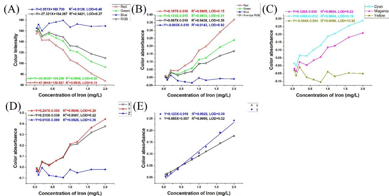
**Fig. S3.** Calibration curves of the Fe(II)-TPTZ system; responses are (A) RGB intensity, (B) RGB colour absorbance, (C) CMY colour absorbance, (D) tristimulus XYZ colour absorbance, and (E) Yxy colour absorbance. The other conditions tested are those shown in Fig. S2.
