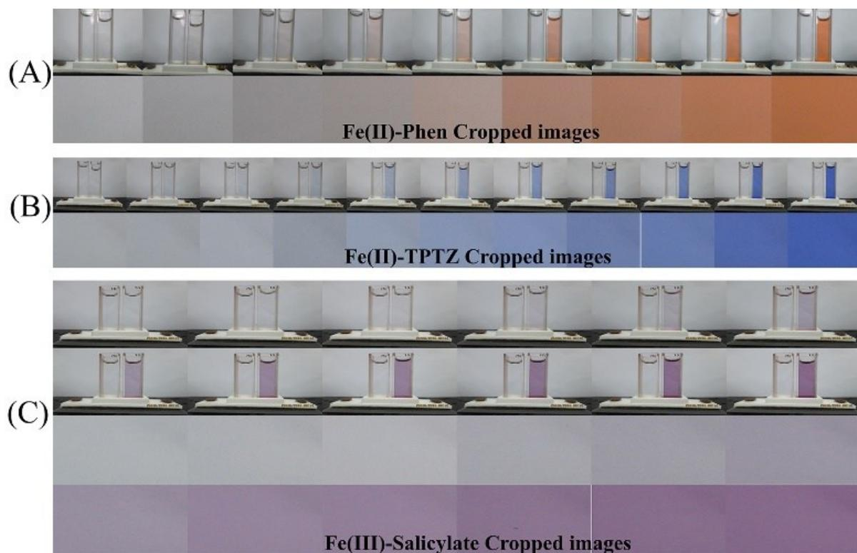
**Fig. S2.** Digital camera images and cropped areas of Fe(II)-phenanthroline standard solutions of 0.0-3.0 mg L<sup>-1</sup> Fe (A), Fe(II)-TPTZ standard solutions of 0.0-2.0 mg L<sup>-1</sup> Fe (B), and Fe(III)-salicylate standard solutions of 0.0-18.0 mg L<sup>-1</sup> Fe (C) obtained according to the recommended procedures. Captured images were arbitrarily compressed to fit into the page margins; however, for image processing, the original uncompressed images were used.
