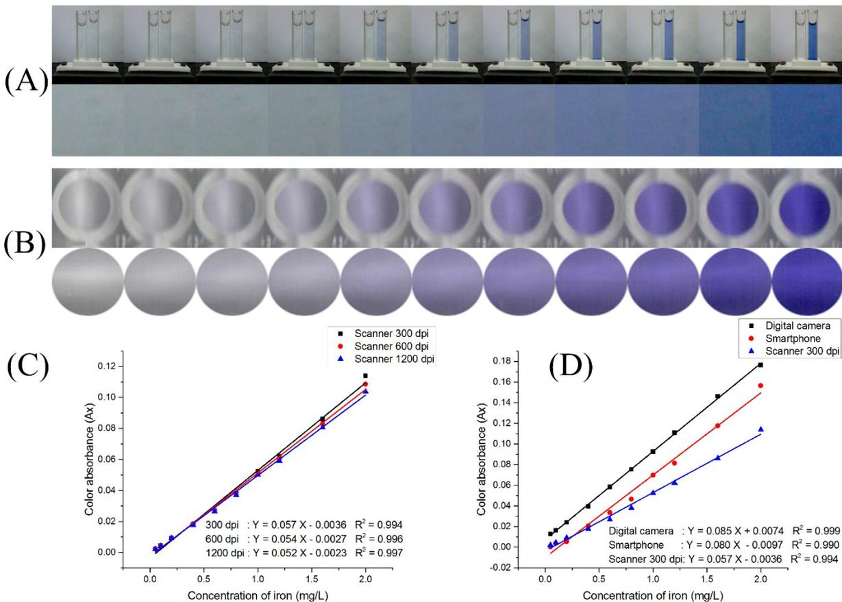
**Fig. S5.** Digital images and cropped images of Fe(II)-TPTZ standard solutions ( $0.0-2.0 \text{ mg L}^{-1}$  Fe). Images were captured using (A) a Sony Xperia E smartphone with a 3.15 MP camera and (B) the scanner of HP LaserJet Pro M1536dnf MF printer at 1200 dpi. Calibration graphs based on images from the desktop scanner at 300, 600 and 1200 dpi (C) and from different image-capturing devices (D). The other conditions tested are those shown in Fig. S2.
