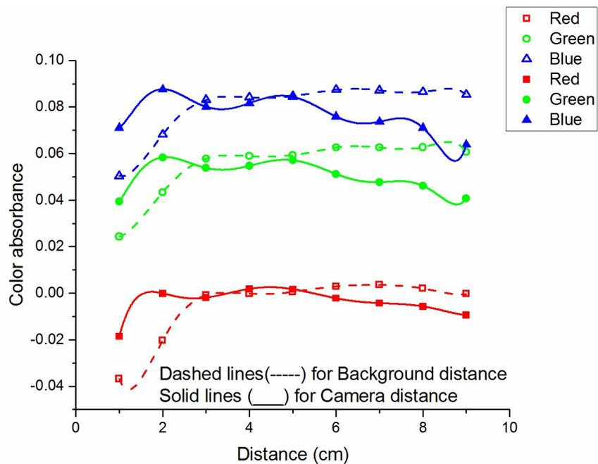
**Fig. S1.** Effects of the cuvette-background diffuser distance (dotted lines) and camera-cuvette distance (solid lines) on the colour absorbances of the Fe-phenanthroline system.
