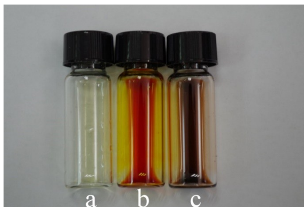
Fig. S1 Images of solutions: (a) Spiro-OMeTAD in chlorobenzene (60 mM), (b) \text{FeCl}_3 in acetonitrile (100 mg/ml), and (c) adding solution b (8 \mu\text{L} ) into solution a (100 \mu\text{L} ).
