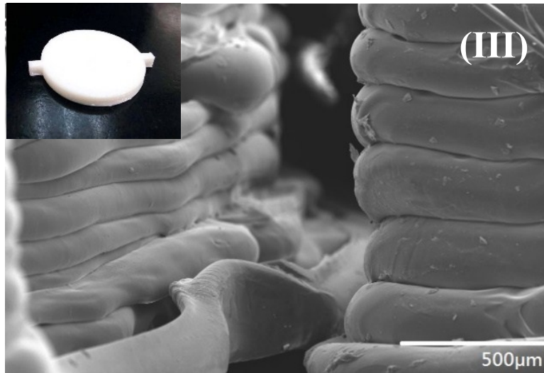
Figure S1 (I) DSC, (II) TGA and (III) SEM results of PLA materials used for the 3D printing
