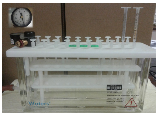
Figure S1: A typical Solid Phase Extraction (SPE) Vacuum Manifold.
