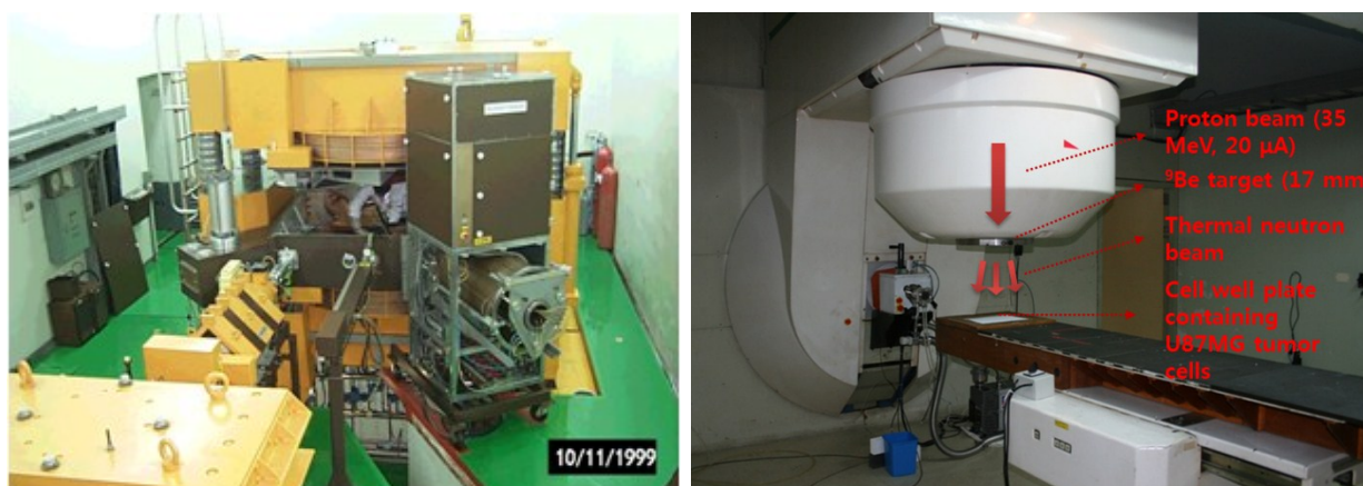
Fig. S5 The MC50 cyclotron (left) and thermal neutron beam irradiation (right) facilities at the Korea Institute of Radiological & Medical Science.
