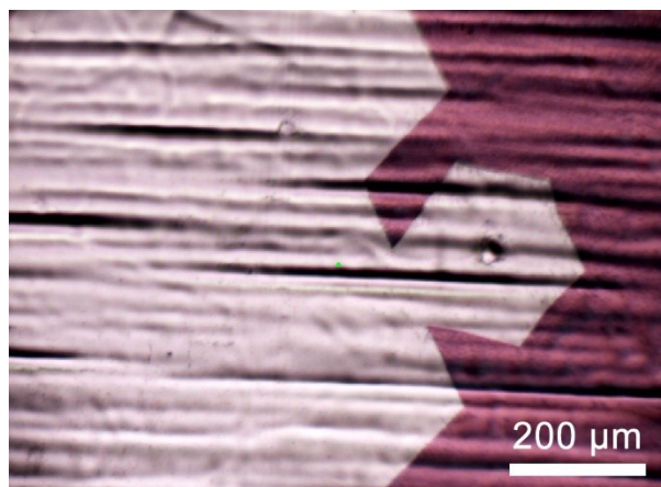
Fig. S2. Growth of aHGDs with prolonged annealing process by H 2 . The results show that the alignment of graphene domains does not change by the H 2 annealing, indicating that the surface monocrystallization maintains even with the H 2 annealing process.
