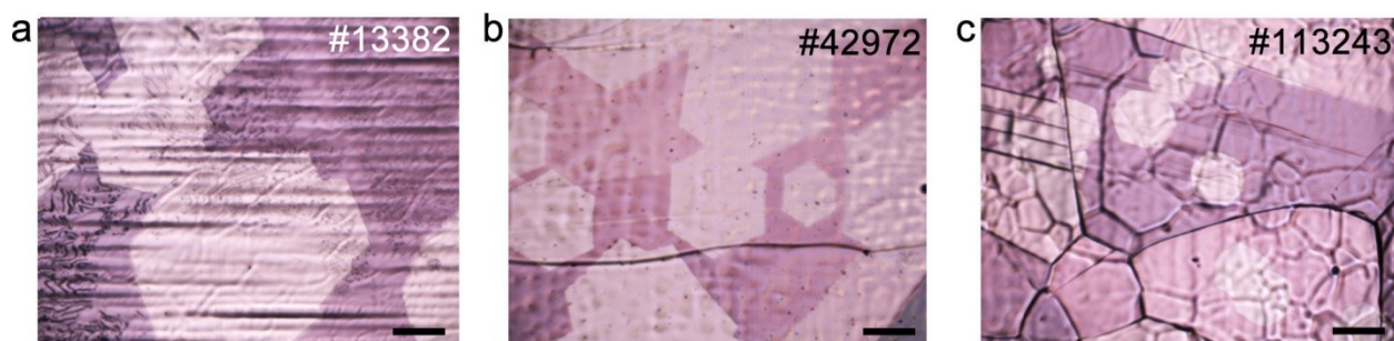
Fig. S1. Growth of aHGDs on different types of commercial Cu foils using oxide-assisted surface monocrystallization. Cu foil product numbers: #13382 and #42972 from Alfa Aesar China Chemical Co., Ltd., #113243 from Nilaco Co., Ltd. All scale bars: 200 \mu\text{m} .
