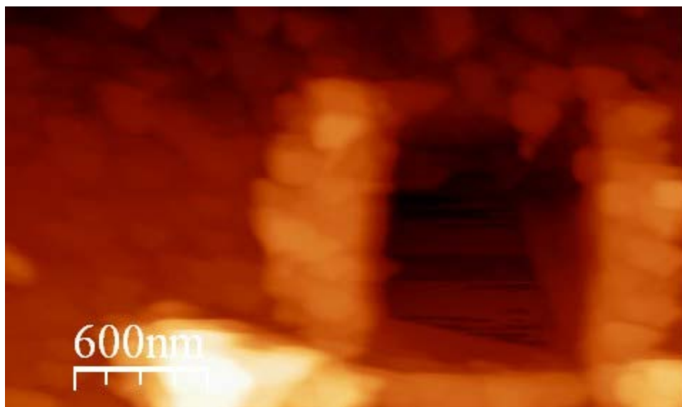
Figure S3. AFM (with scratched region) of a ferrocene-functionalized PPBD film deposited from water (60 min.) on ITO. Scratch depth 60 nm.
