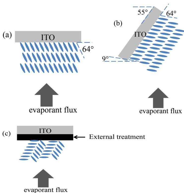
Fig. S1 Schematic demonstration of co-deposition of ZnPc and PTCBI on ZnPc coated ITO substrate, (a) horizontal substrate and (b) tilted substrate. (c) Face-on ZnPc grains grown on particularly treated ITO substrate. Blue ellipse stands for ZnPc molecules.
