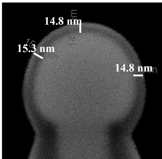
Fig. S2 SEM image of a typical tip after field emission measurement. The semitransparent out layer is the ZnPc/PTCBI bilayer with the thickness of  $\sim 15$  nm, the brighter central part is W-tip.
