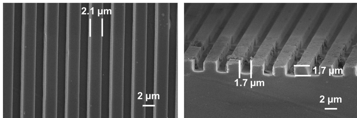
**Figure S5.** Aerial and cross-sectional views of the PDMS mold used in this study.
