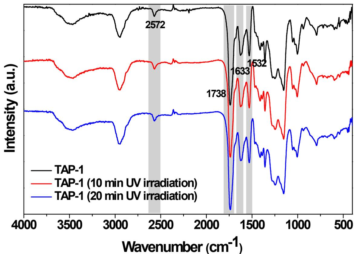
**Figure S2.** FT-IR study of thiol-ene photo-addition in the titanium-containing resin, TAP-1.0.
