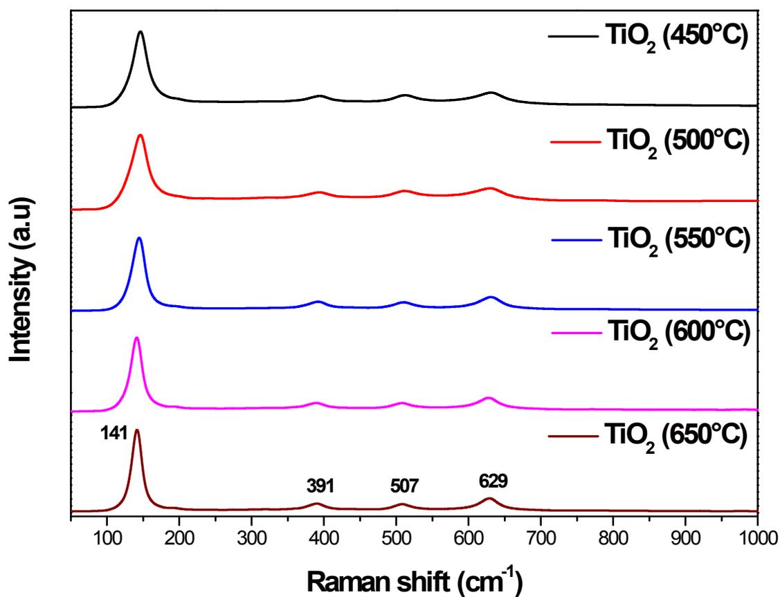
**Figure S4.** Raman spectra of TiO<sub>2</sub> obtained by calcination of photo-cured TAP-0.5 thin films at various temperatures.
