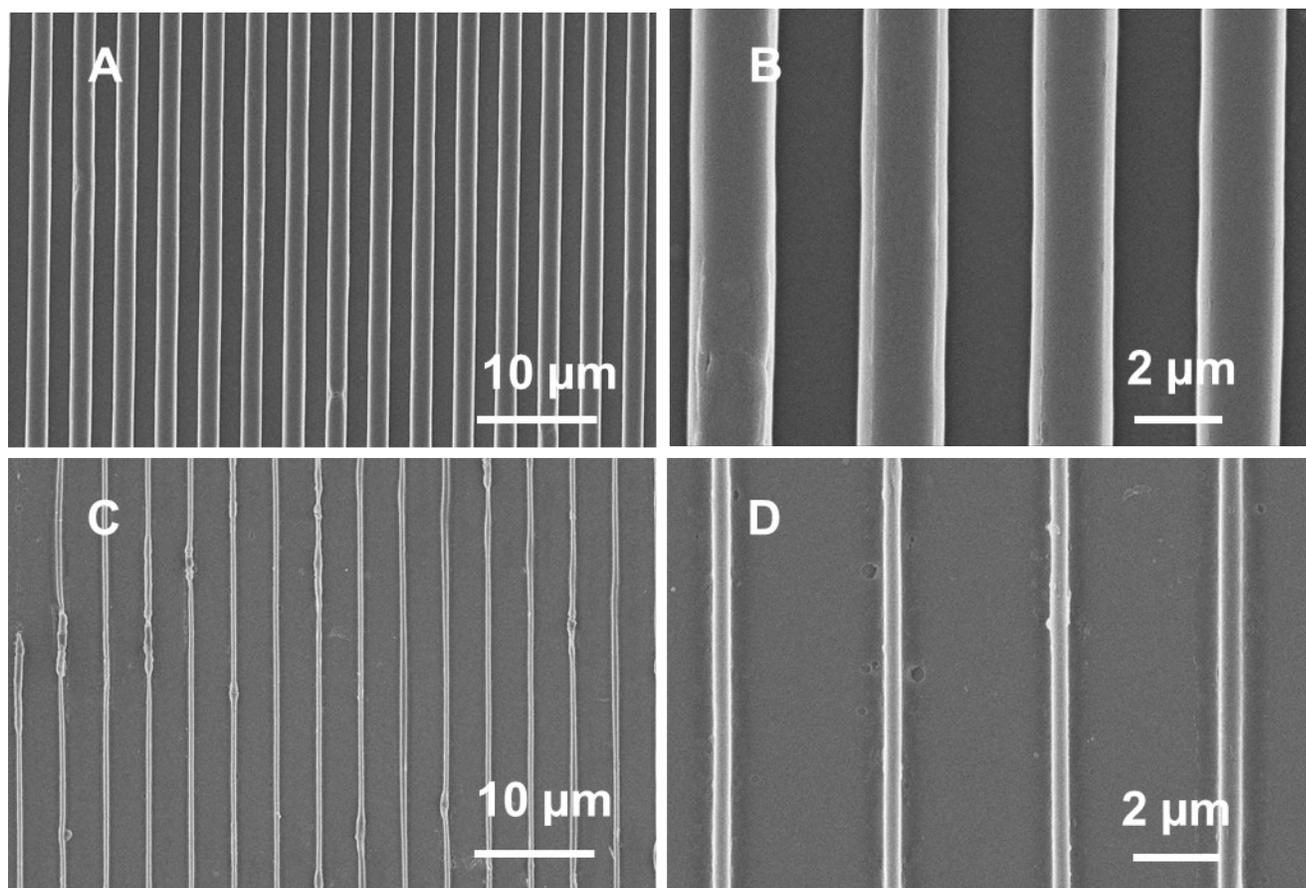
**Figure S6.** FE-SEM images of imprinted lines of  $\text{Ti}(\text{MAEAA})_4$ -based resin (A and B) before and (C and D) after calcination.
