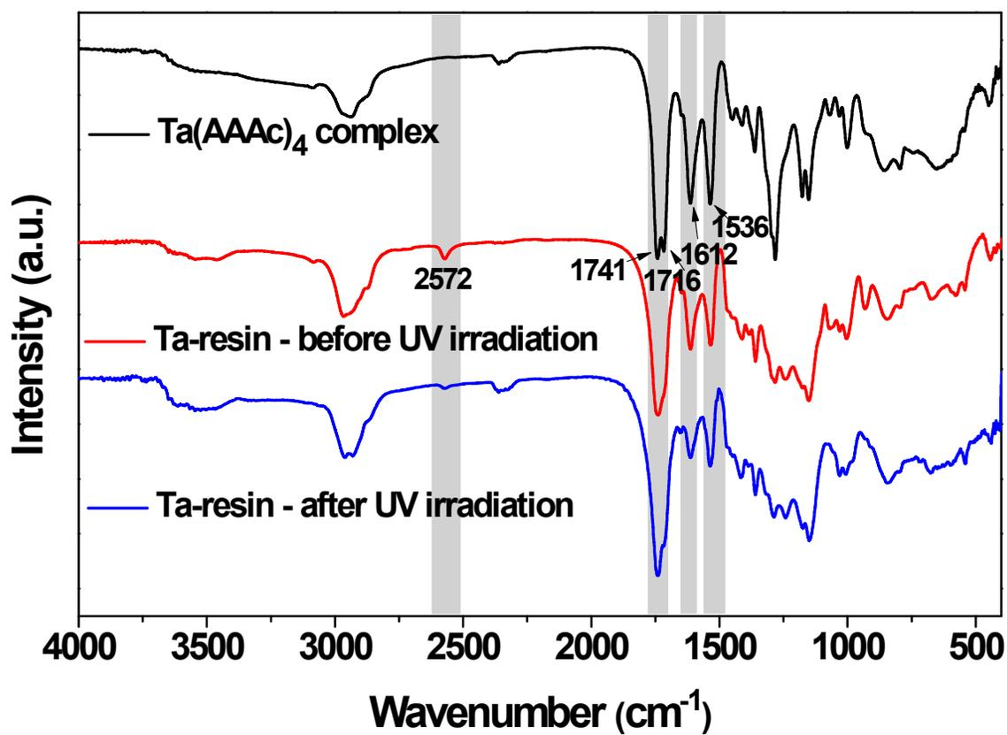
**Figure S7.** FT-IR analysis of Ta(AAac)<sub>4</sub> complex, and tantalum-containing resin before and after UV irradiation to probe the thiol-ene click reaction.
