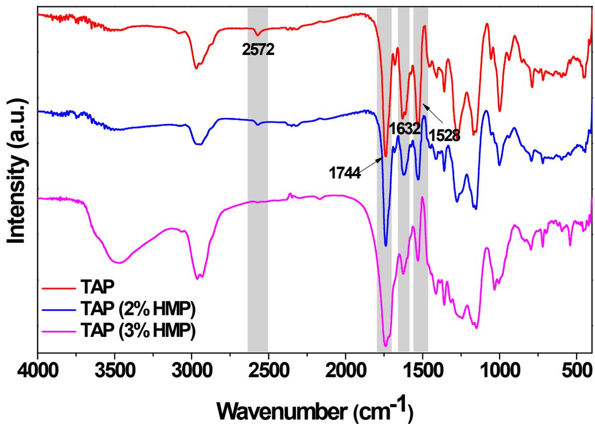
**Figure S3.** FT-IR analysis of TAP-0.5 without and with different amounts of HMP photo-initiator. The optimized loading of the photo-initiator was found to be 3%.
