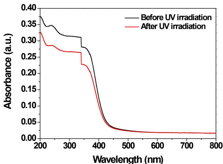
**Figure S1.** UV-visible absorbance spectra of TAP-0.5 thin film (coated over quartz substrate) before and after UV irradiation.
