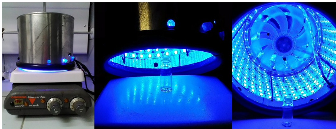
Figure S1. Photochemical set up.
