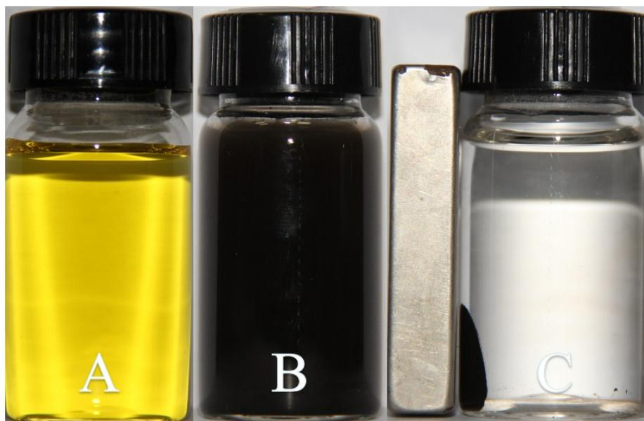
**Figure S7.** (A) The photograph of hexavalent chromium ion (100mg/L) (B) GMFP nanocomposites can be dispersed in water and (C) separated from water using a magnet .
