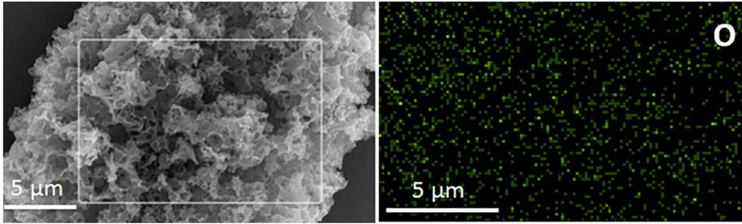
**Figure S1.** SEM image (a) and elemental mapping image (b) of O element for as-obtained porous carbon sample.
