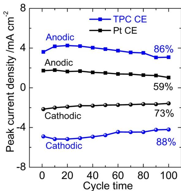
**Figure S3.** The changes in cathodic and anodic peak current densities of redox couple ( $I_3^-/I^-$ ) on the TPC and Pt electrode in CV measurement during the 100 scanning cycles.
