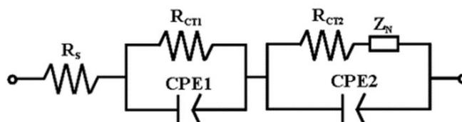
**Scheme S2.** The equivalent circuit for fitting data in Figure 6b.  $R_{ct1}$ : the charge-transfer resistance at the interface of the counter electrode and the liquid electrolyte;  $R_{ct2}$ : charge transfer resistance at the  $TiO_2$ /dye/electrolyte interfaces;  $Z_N$ : Nernst diffusion resistance of the redox couple within the electrolyte; CPE1 and CPE2: double-layer capacitances.
