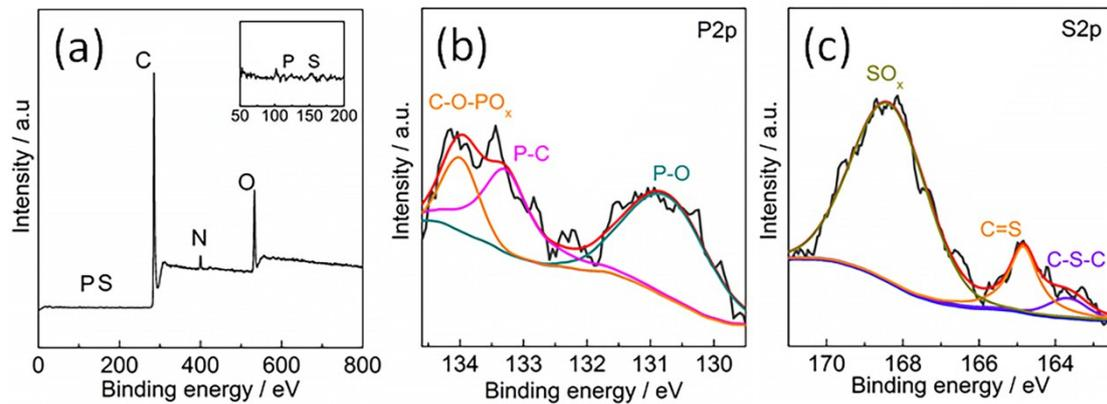
**Figure S2.** (a) The XPS survey spectra of as-obtained porous carbon sample with high resolution XPS spectra of (b) P 2p and (c) S2p element.
