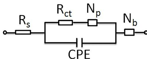
**Scheme S1.** The equivalent circuit for fitting experimental data in Figure 5b.  $R_s$ : Series resistance;  $R_{ct}$ : charge transfer resistance; CPE: double-layer capacitance;  $N_p$ : Nernst diffusion impedance within the electrode pores;  $N_b$ : bulk Nernst diffusion impedance in the electrolyte.
