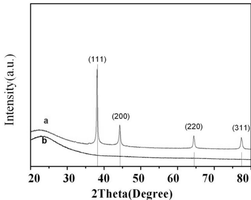
**Figure S8.** XRD patterns obtained for (a) Ag@WMSs-NNN and (b) WMSs-NNN nanoparticles.
