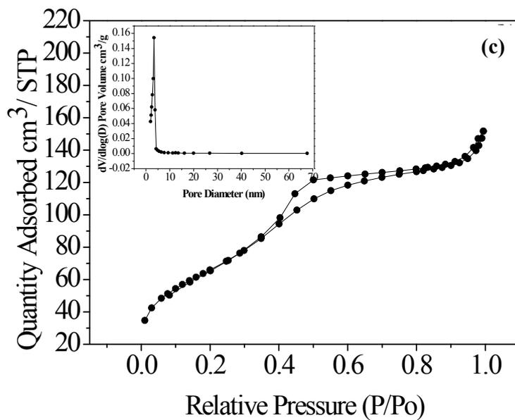
**Figure S5.** N<sub>2</sub> adsorption/desorption isotherms and pore size distribution of WMSs-NNN nanoparticles.
