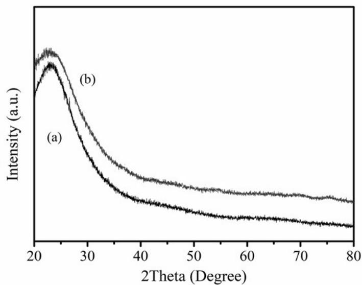
**Figure S3.** XRD patterns obtained for (a) Ag@WMSs-N and (b) WMSs-N nanoparticles.
