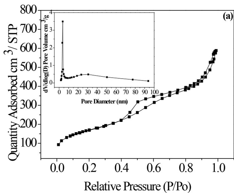
**Figure S2.** N<sub>2</sub> absorption/desorption isotherms and pore size distribution of WMSs-N nanoparticles.
