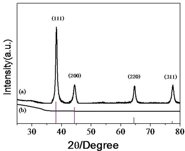
**Figure S6.** XRD patterns obtained for (a) Ag@WMSs-N2 and (b) WMSs-N2 nanoparticles.
