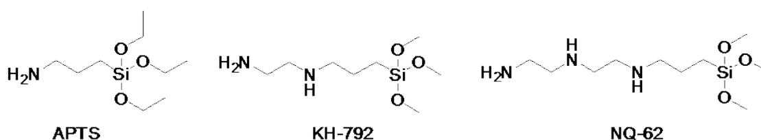
**Figure S1.** The structural formulas of APTES, KH-792 and NQ-62.
