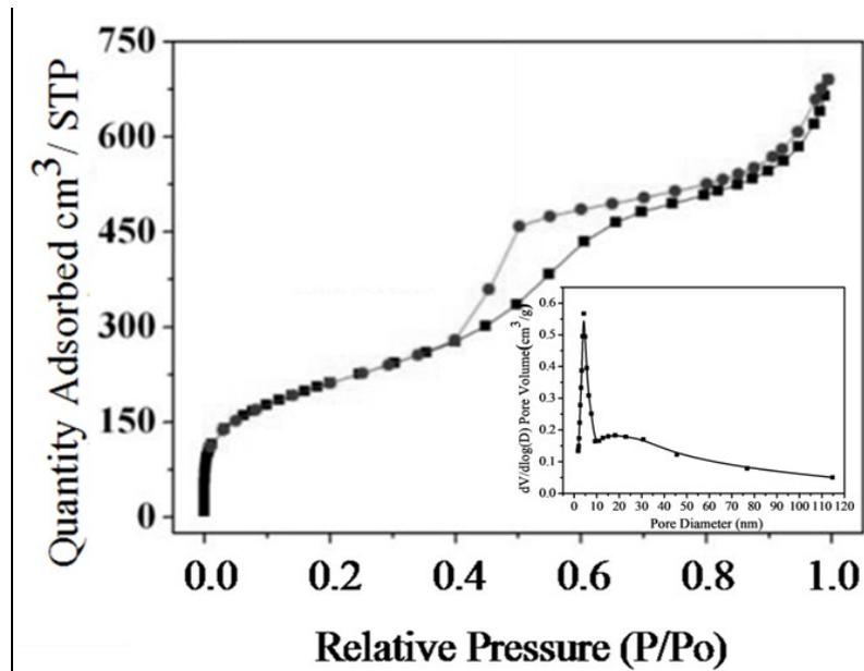
**Figure S4.** N<sub>2</sub> adsorption/desorption isotherms and pore size distribution of WMSs-NN nanoparticles.
