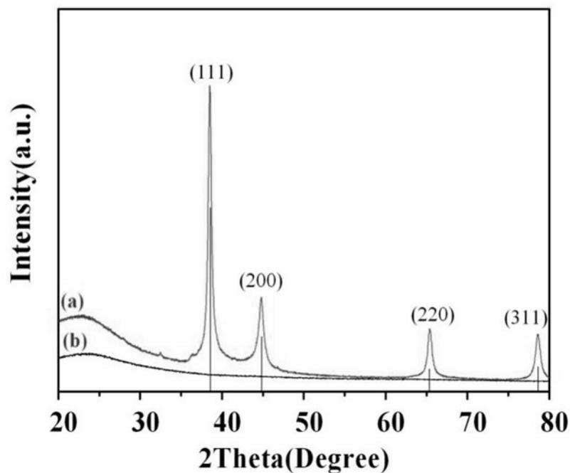
**Figure S7.** XRD patterns obtained for (a) Ag@WMSs-NN and (b) WMSs-NN nanoparticles.
