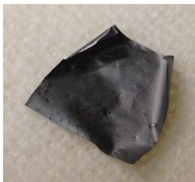
Fig. S1. Image of the 10 \mu\text{m} thick RGO film. We straightened and cut the film to 10 mm \times 10 mm before we applied it as a barrier layer in the plasticized PVC films.
