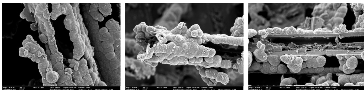
Fig. S5 SEM images of the polymer isolated after a reaction time of 90 min and washed with methanol.
