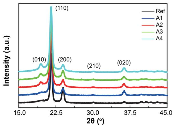
Fig. 3S XRD curves of HDPE samples recovered after different D-ECAP processes.
