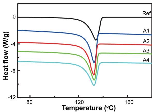
Fig. 2S DSC curves of HDPE samples recovered after different D-ECAP processes.
