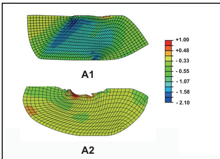
Fig. 1S FEM results of A1 and A2 D-ECAP processes.
