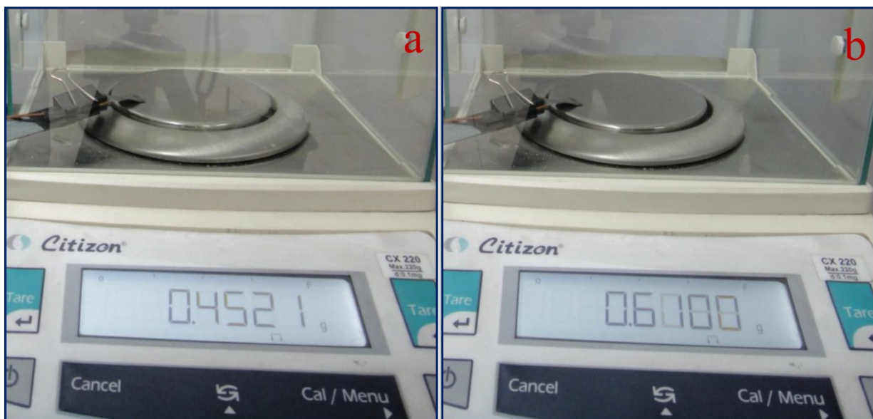
Supplementary Figure 2. Load characterization of (a) SPEES/PVDF/Pt and (b) SPEES/PVDF/SGO/Pt based IPMC membrane actuators.
