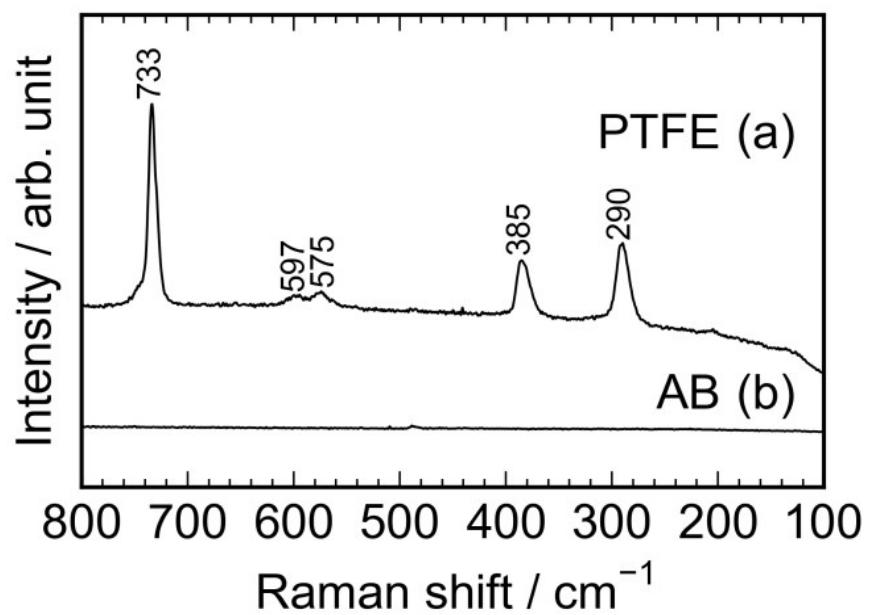
Fig. S5 Raman spectra for (a) PTFE and (b) AB.
