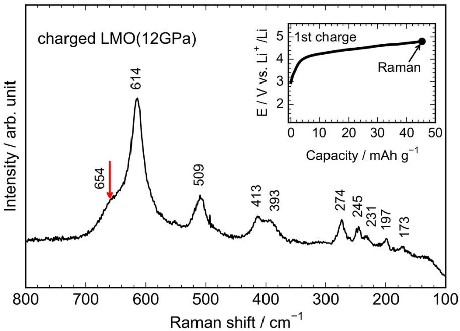
Fig. S3 *Ex situ* Raman spectrum of the charged LMO(12GPa) sample. The inset indicates its charge curve up to 4.8 V. The Raman band at  $654 \text{ cm}^{-1}$  is originated from  $\text{Li}_x\text{Mn}_2\text{O}_4$  spinel phase.
