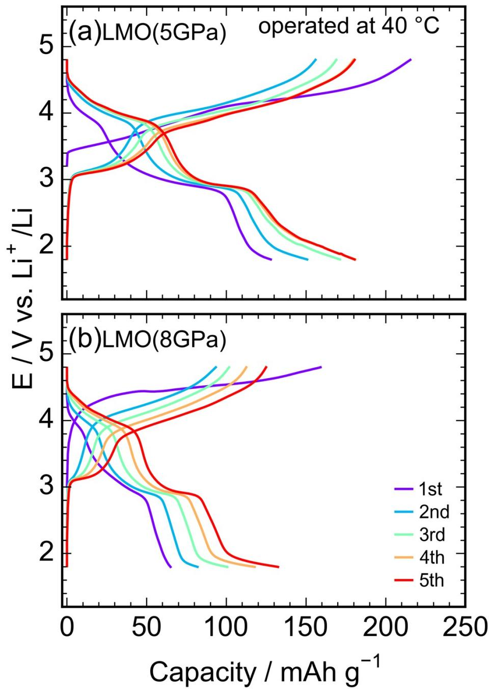
Fig. S2 Charge and discharge curves of the lithium cells with the (a) LMO(5GPa) and (b) LMO(8GPa) samples. The cells were operated at a temperature of 40 °C.
