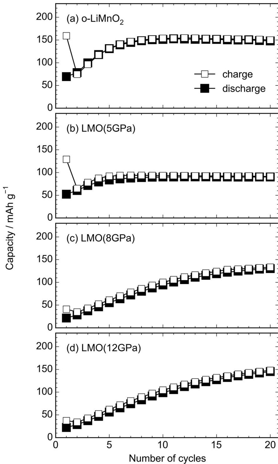
Fig. S1 Cycle performances at 25 °C of the (a) o-LiMnO<sub>2</sub>, (b) LMO(5GPa), (c) LMO(8GPa), and (d) LMO(12GPa) samples. Open and closed squares indicate charge and discharge capacities, respectively.
