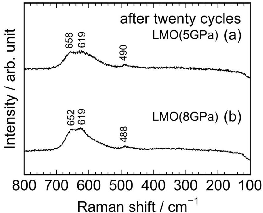
Fig. S4 *Ex situ* Raman spectra of the cycled (a) LMO(5GPa) and (b) LMO(8GPa) samples. Raman spectra were taken at the discharged state indicated by the red arrows in Figs. 5b and 5c in the text.
