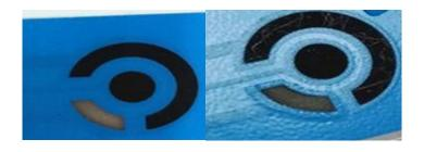
Fig 3S. Photos of screen printed electrodes before (left) and after (right) deposition of rGO/PANi film: The rGO/PANi film is porous and in dark color.
