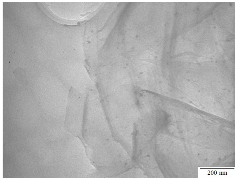
Fig. S1 TEM image of GeQD/NGr nanocomposite.
