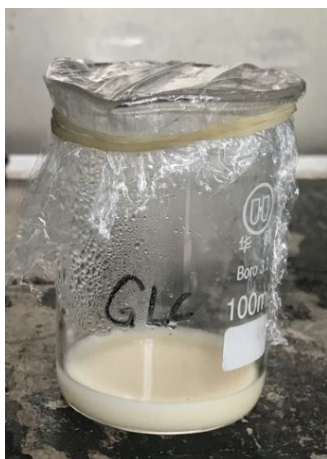
Fig. S3 The crosslinked network formed by mixing of glucose and glutaraldehyde solution.
