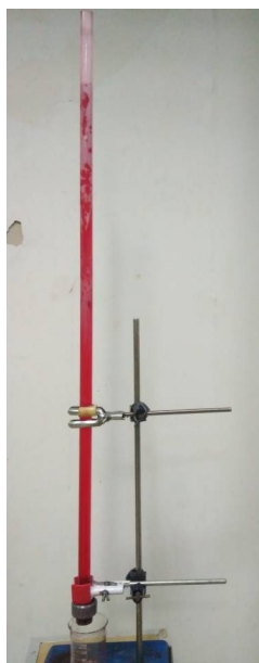
Fig. S4 A modified filter paper with an area of 2.54 \text{ cm}^2 could support a column of toluene 0.72 m, a column of hexane 0.83 m, and a column of petroleum ether 0.90 m in height, respectively.
