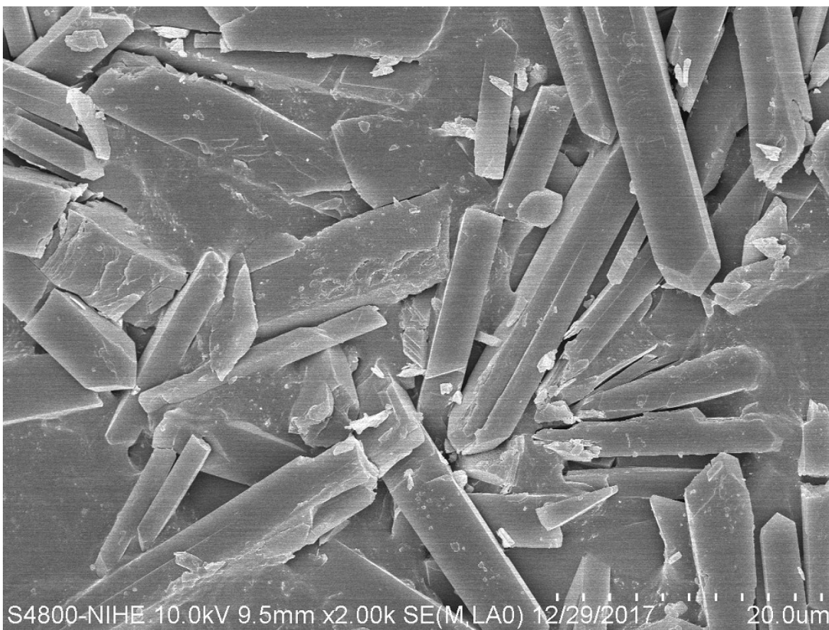
Fig. S2. SEM micrograph of Cu 2 (OBA) 2 (BPY).
