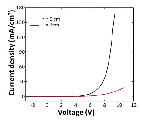
Figure S1 *J*-*V* characteristics of TOLEDs with DBR under different mechanical bending radius, r = 5 and 3 cm.
