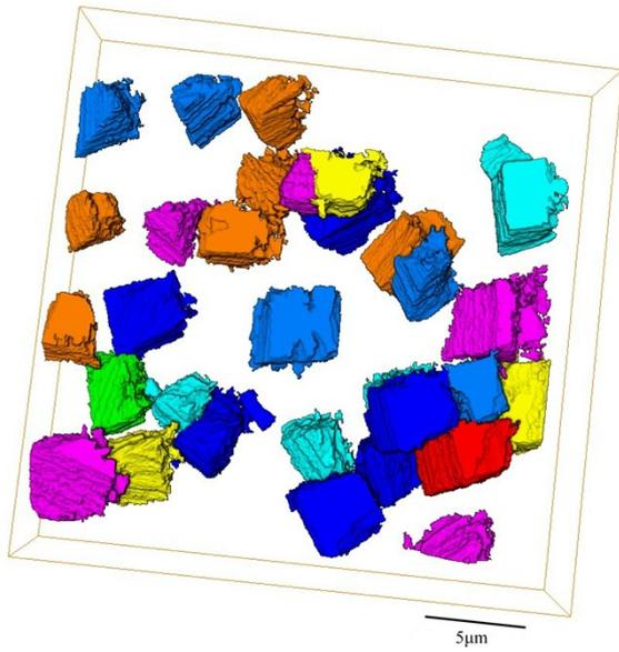
**Figure S2** Volume reconstruction obtained by automatic segmentation. (Colors are randomly assigned to each SAPO-34 particle by labeling module of Avizo software.)
