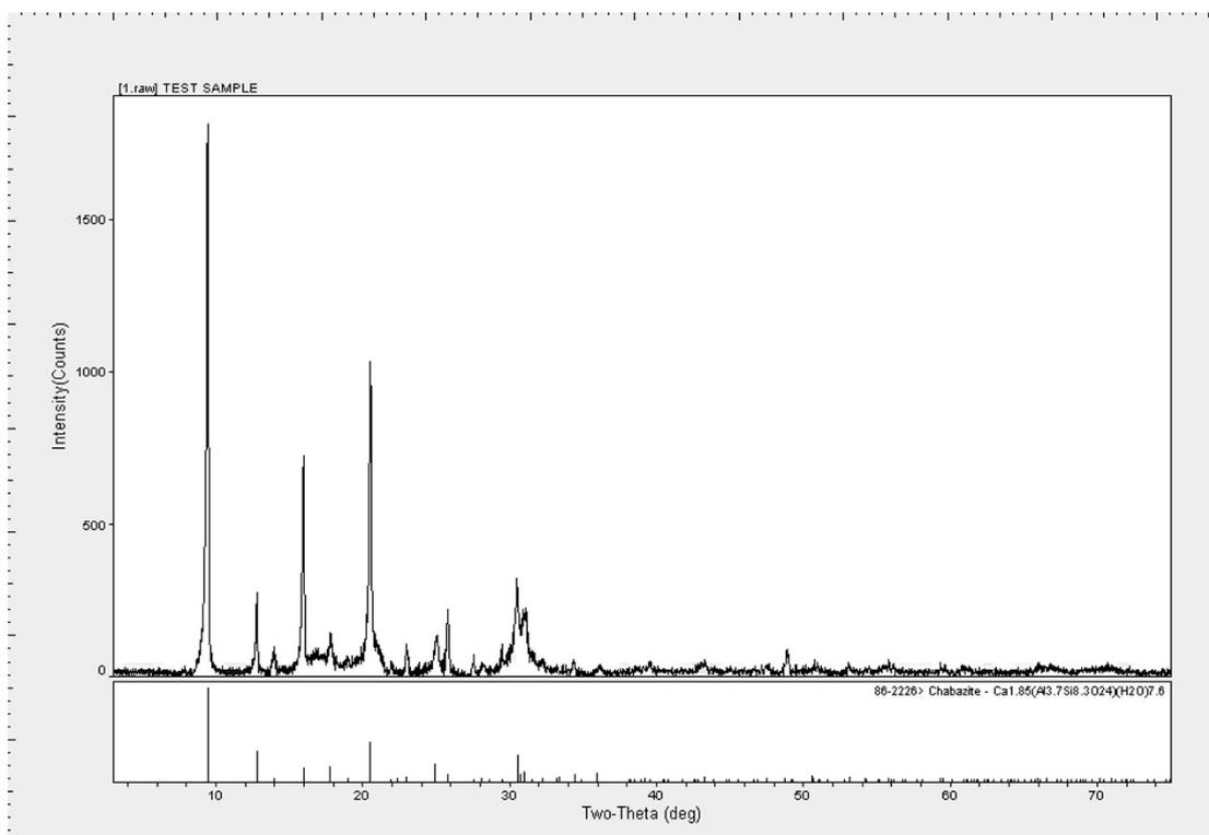
**Figure S4** Powder X-ray Diffraction (XRD) pattern of the SAPO-34 sample
