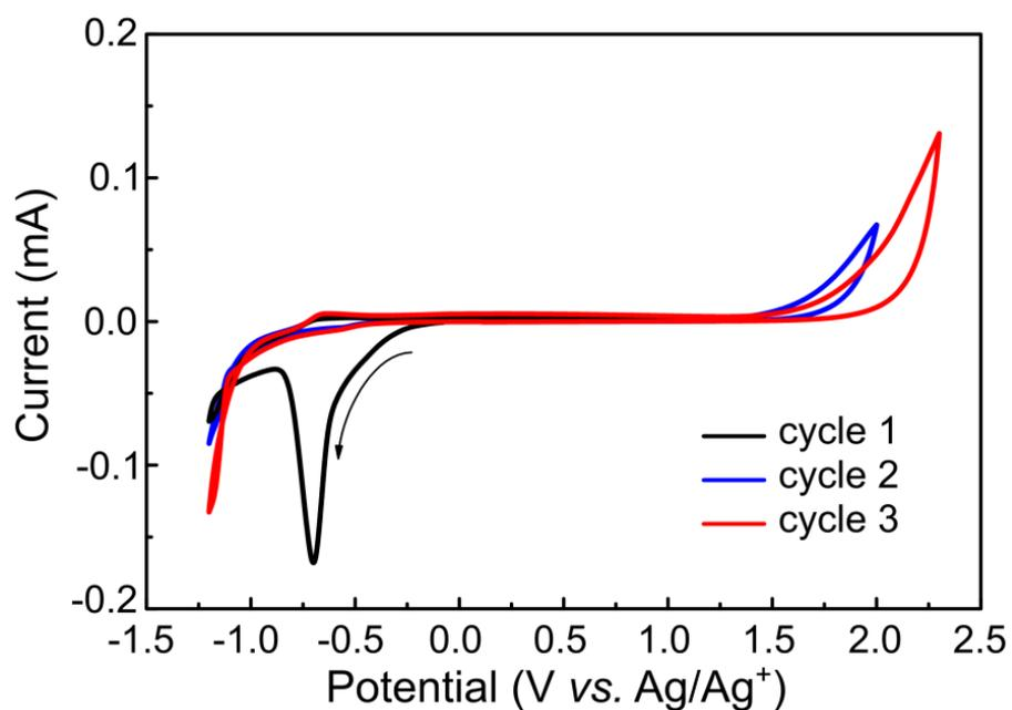
SI 3: a) Cyclic voltammogram at  $10 \text{ mV s}^{-1}$  of a  $\text{MoO}_3$  film on ITO in  $1 \text{ mol L}^{-1} \text{Mg}(\text{ClO}_4)_2$  in PC. The cathodic peak shows the irreversible intercalation of  $\text{Mg}^{2+}$  in  $\text{MoO}_3$ .
