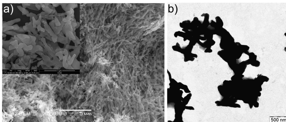
SI 4: TEM images of  $\text{MoS}_2$  obtained through heating from room temperature to  $800 \text{ }^\circ\text{C}$  at  $30 \text{ }^\circ\text{C}/\text{min}$  under  $5 \text{ } \%/95 \text{ } \% \text{ H}_2/\text{N}_2$  ( $96 \text{ mL min}^{-1}$ ).  $\text{H}_2\text{S}$  was streamed after the temperature reached  $400 \text{ }^\circ\text{C}$ . The sample was treated at  $800 \text{ }^\circ\text{C}$  for 30 min.
