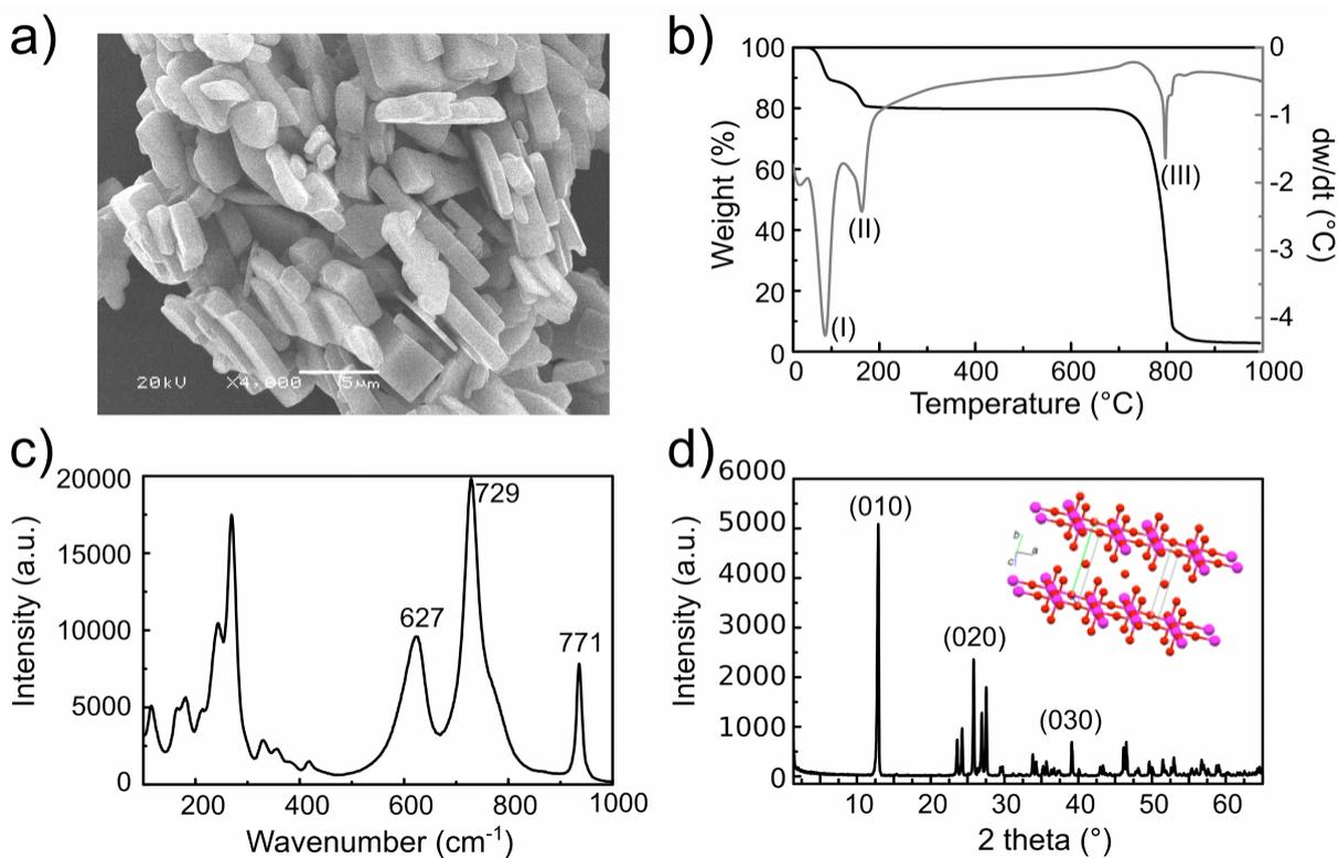
SI 1: Characterization of the precursor  $\text{MoO}_3 \cdot 2\text{H}_2\text{O}$ : a) SEM image, b) TG-DTA curves, c) Raman spectrum and d) XRD pattern.
