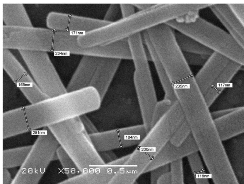
SI 2: Diameter measurement of SEM images of as-prepared  $\text{MoO}_3$  nanoribbons.
