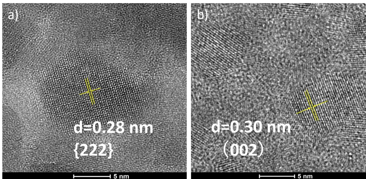
S1) HR TEM images and d-spacing measurements for a) Cu<sub>6</sub>PS<sub>5</sub>Cl and b) Cu<sub>3</sub>PS<sub>4</sub>. These measurements agree with standard crystallography data
