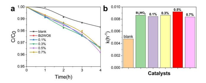
Fig S2 Comparison of different photocatalysts for photodegradation of phenol for 10 ppm
