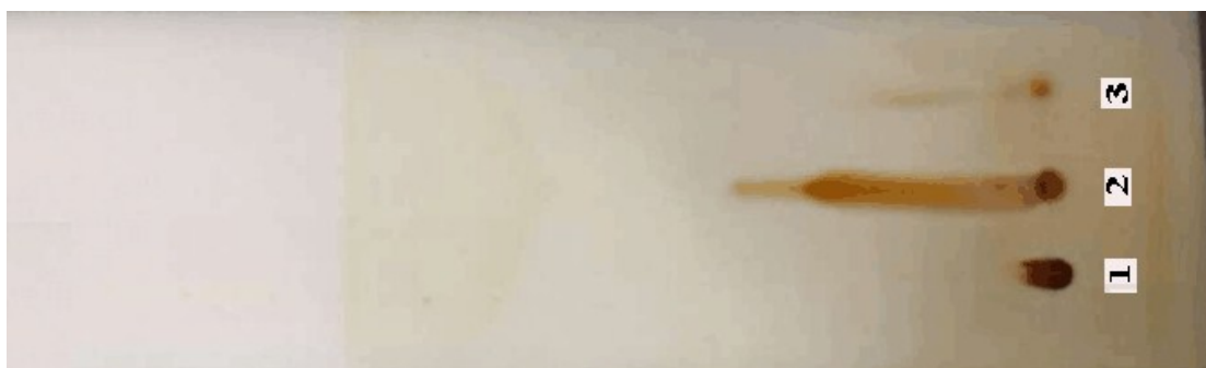
Fig. S7 Thin-Layer Chromatography (TLC) spectra of NHS-PEG-MAL-G5.0 PAMAM: chloroform-methanol (5: 1, v/v) was applied as TLC developing solvent for the separation of different components. The iodine steam was selected as chromogenic agent. Hydroxyl-terminated G5.0 PAMAM (lane 1), NHS-PEG-MAL-G5.0 PAMAM (lane 2) and MAL-PEG 3400 -NHS (lane 3) were shown in this diagram, respectively.
