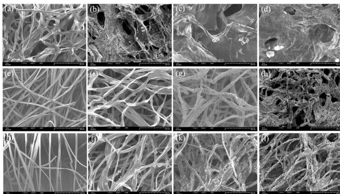
**Figure S7** SEM images of materials degradation experiment. (a) – (d) Ca-Alg fibrous scaffolds; (e) – (h) the commercial wound dressing No.1; (i) – (l) the commercial wound dressing No.2; (a), (e), (i) the initial of test; (b), (f), (j); after 2 h absorption in PBS buffer; (c), (g), (k) after 12 h absorption in PBS buffer; (d), (h), (l) after 48 h absorption in PBS buffer.
