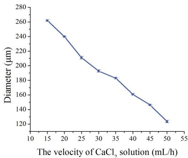
**Figure S4** The mean diameter of Ca-Alg fibers prepared in different velocity of  $\text{CaCl}_2$  solution.
