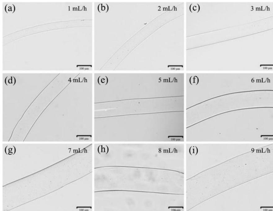
**Figure S1** The morphology of Ca-Alg fibers prepared in different velocity of Na-Alg solution. (The bar is 100  $\mu\text{m}$ ).
