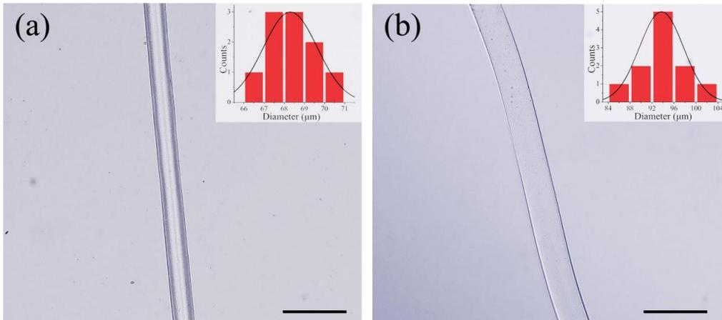
**Figure S5** The morphology of Ca-Alg fibers before water absorption (a) and after water absorption (b). (The bar is 200  $\mu\text{m}$  )
