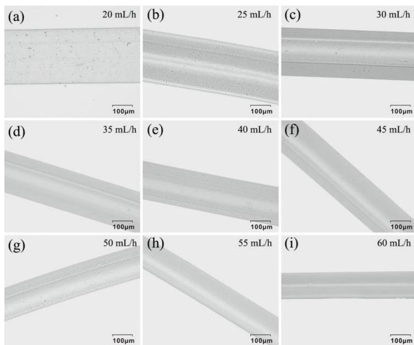
**Figure S3** The morphology of Ca-Alg fibers prepared in different velocity of  $\text{CaCl}_2$  solution. (The bar is  $100\ \mu\text{m}$ ).
