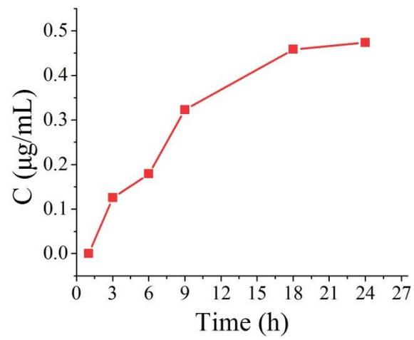
**Figure S8** The curve of silver ions release of the Ca-Alg fibrous scaffold loaded with AgNPs.
