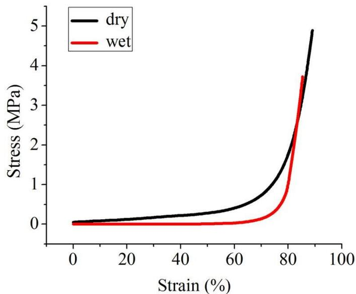
**Figure S6** Stress-strain curve for the Ca-Alg fibrous scaffold (dry and wet).
