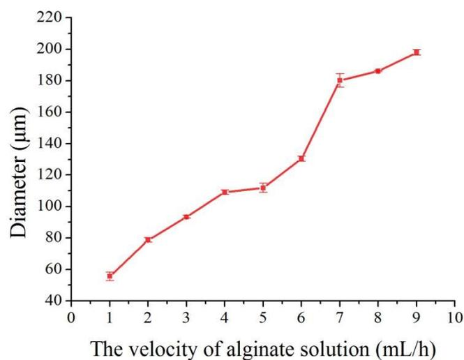
**Figure S2** The mean diameter of Ca-Alg fibers prepared in different velocity of Na-Alg solution.
