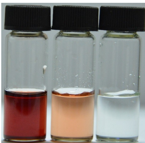
Fig. S3. Visible change in color of L3 in DMSO solution on the addition of 10 equiv. of fluoride ions: (a) 1 \times 10^{-2} M of L3 , (b) 1 \times 10^{-3} M of L3 , (c) 1 \times 10^{-4} M of L3 (a, b, and c, left to right).
