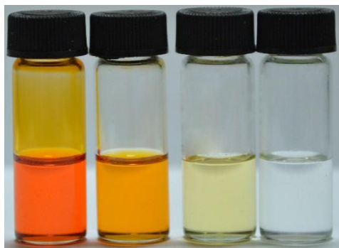
Fig. S1. Visible change in color of L1 in DMSO solution on the addition of 10 equiv. of fluoride ions: (a) 1 \times 10^{-2} M of L1 ; (b) 1 \times 10^{-3} M of L1 ; (c) 1 \times 10^{-4} M of L1 ; (d) 1 \times 10^{-5} M of L1 (a, b, c and d, left to right).
