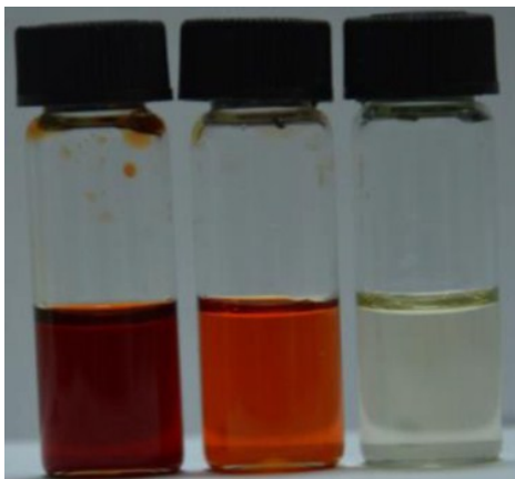
Fig. S2. Visible change in color of L2 in DMSO solution on the addition of 10 equiv. of fluoride ions: (a) 1 \times 10^{-2} M of L2 ; (b) 1 \times 10^{-3} M of L2 ; (c) 1 \times 10^{-4} M of L2 (a, b, and c, left to right).
