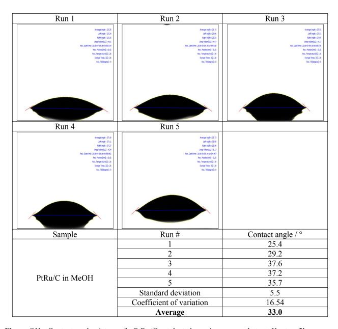
**Figure S1b:** Contact angle picture of a PtRu/C catalyst slurry drop on a substrate Kapton film; PtRu/C in methanol (MeOH) dispersion.
