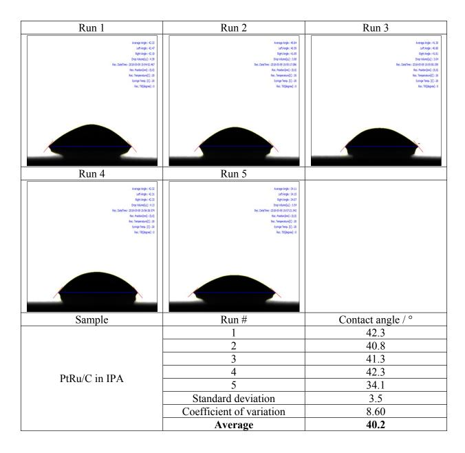
**Figure S1a:** Contact angle picture of a PtRu/C catalyst slurry drop on a substrate Kapton film; PtRu/C in isopropyl alcohol (IPA) dispersion.
