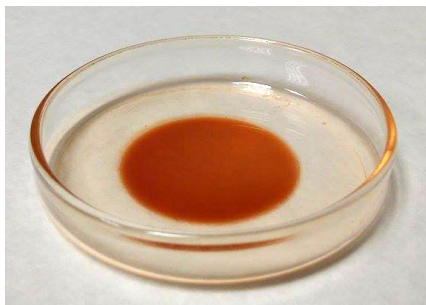
Figure S2. Picture of a flexible highly piezo resistive bilayer film-based support consisting of polycarbonate/ 001 oriented polycrystalline layer of \alpha -(BEDT-TTF) 2 I 3 . [6] The conducting layer is self-assembled at the central part of the film.
