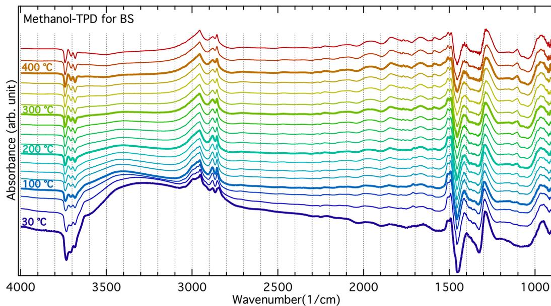
Figure S12: Infrared spectra collected during temperature programmed desorption of methanol from the BS sample ramping the temperature from 30 to 450 °C.
