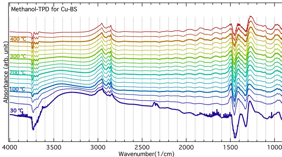
Figure S13: Infrared spectra collected during temperature programmed desorption of methanol from the Cu-BS sample ramping the temperature from 30 to 450 °C.
