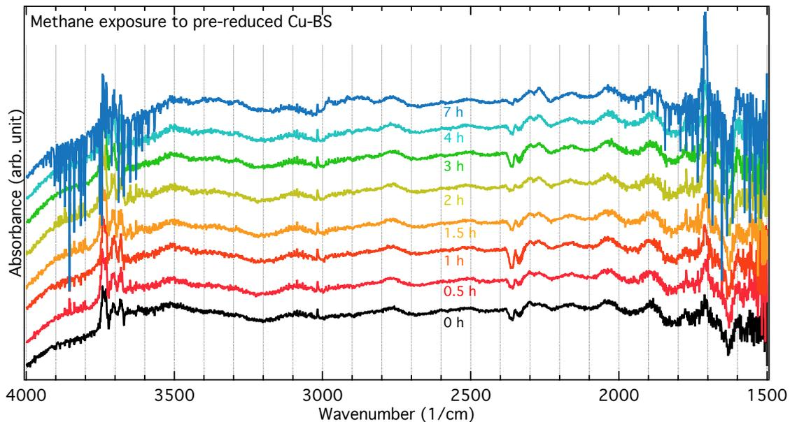
Figure S10: Infrared spectra for pre-reduced Cu-BS exposed to methane at 250 °C during 0 to 7 h. All spectra were recorded in Ar.
