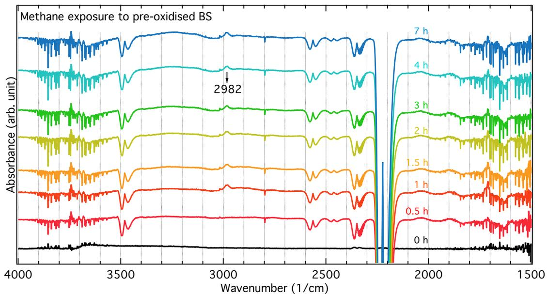
Figure S5: Infrared spectra for pre-oxidised BS exposed to methane at 250 °C during 0 to 7 h. The spectrum at 0 h was taken in presence of 500 ppm of  $N_2O$  whereas the remaining spectra were recorded in Ar.
