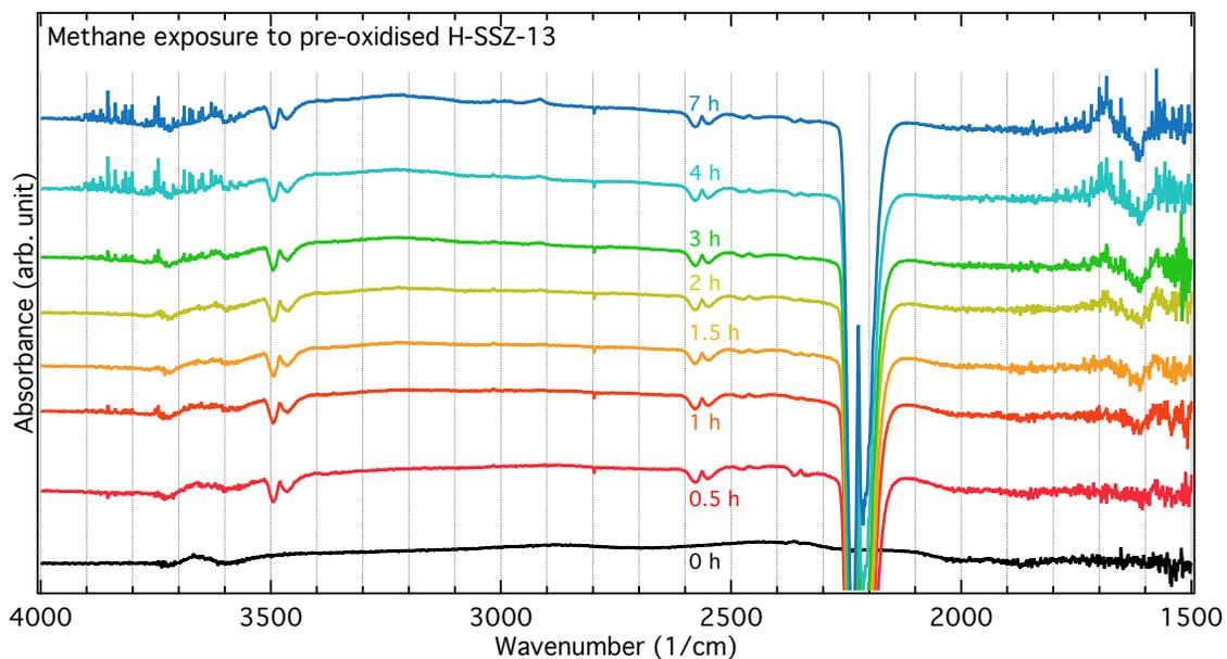
Figure S7: Infrared spectra for pre-oxidised H-SSZ-13 exposed to methane at 250 °C during 0 to 7 h. The spectrum at 0 h was taken in presence of 500 ppm of N<sub>2</sub>O whereas the remaining spectra were recorded in Ar.
