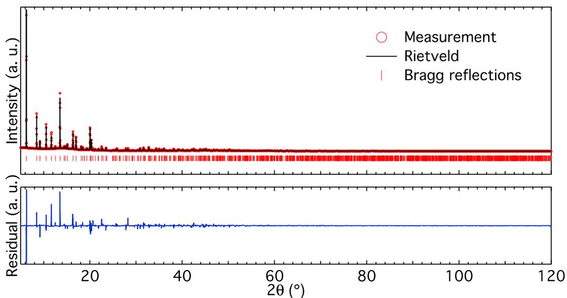
Figure S2: High-resolution X-ray diffractogram (upper panel) and Rietveld refinement (lower panel) for the BS sample.
