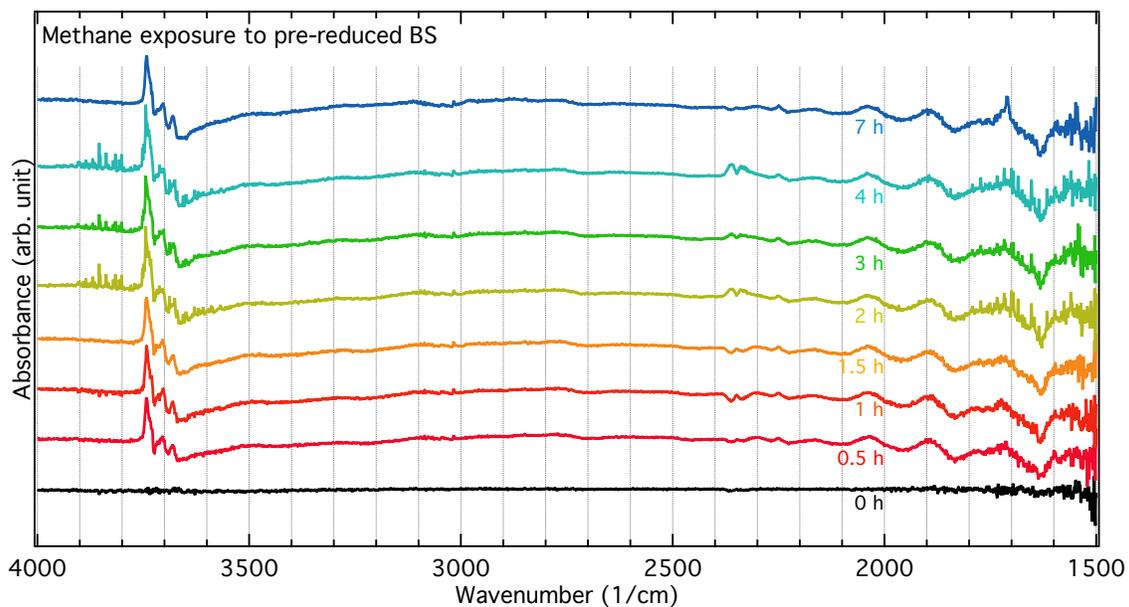
Figure S6: Infrared spectra for pre-reduced BS exposed to methane at 250 °C during 0 to 7 h. All spectra were recorded in Ar.
