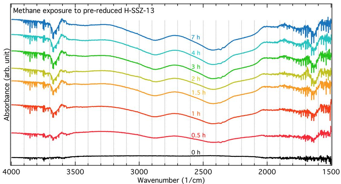
Figure S8: Infrared spectra for pre-reduced H-SSZ-13 exposed to methane at 250 °C during 0 to 7 h. All spectra were recorded in Ar.
