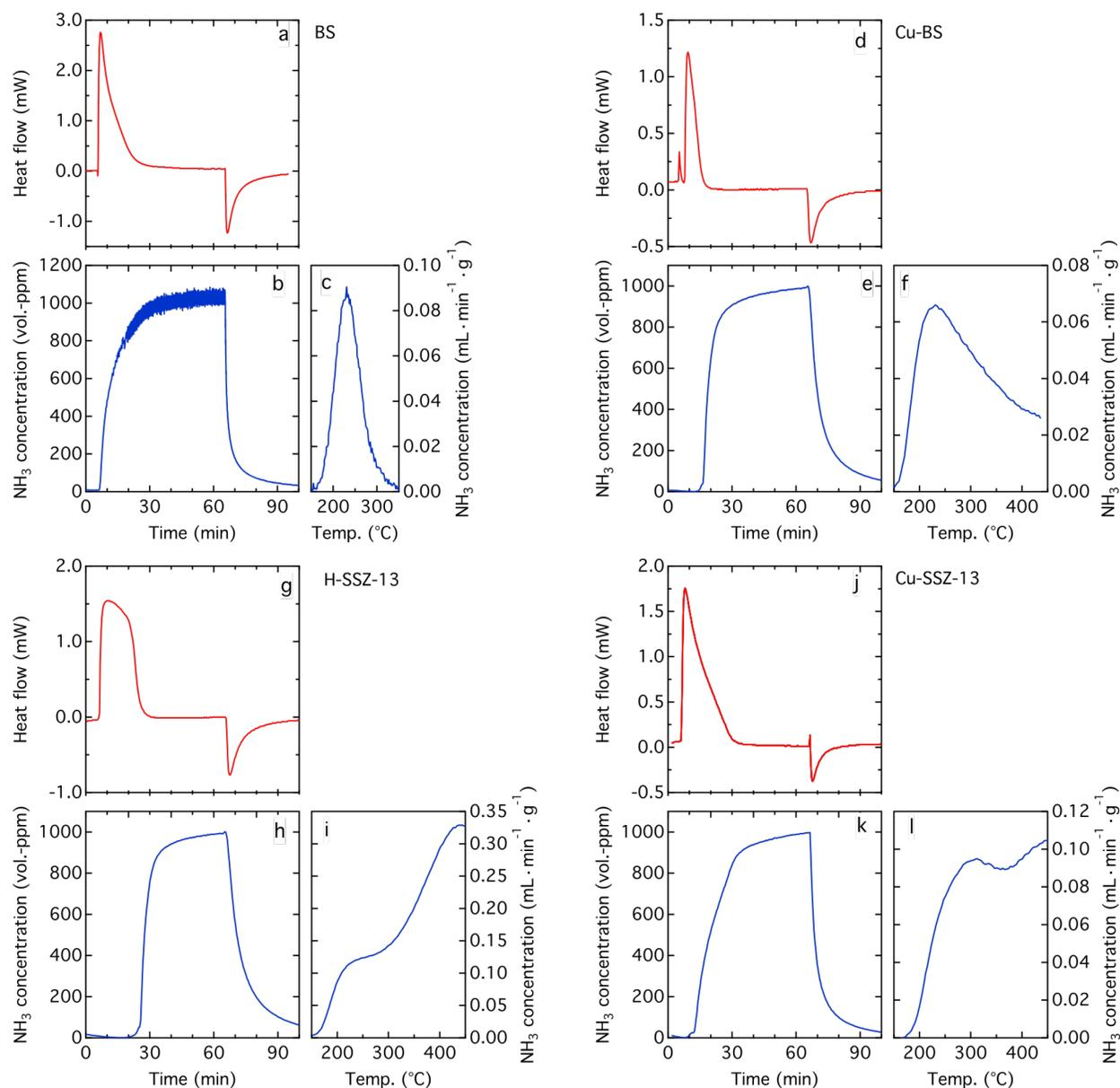
Figure S3: Thermogram (a, d, g, j) and ammonia mass spectrometer signal during  $\text{NH}_3$  adsorption (b, e, h, k), and  $\text{NH}_3$  desorption profile during linear heating (c, f, i, l) of the BS, Cu-BS, H-SSZ-13 and Cu-SSZ-13 sample.
