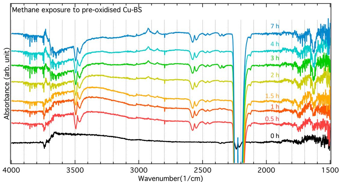
Figure S9: Infrared spectra for pre-oxidised Cu-BS exposed to methane at 250 °C during 0 to 7 h. The spectrum at 0 h was taken in presence of 500 ppm of N<sub>2</sub>O whereas the remaining spectra were recorded in Ar.
