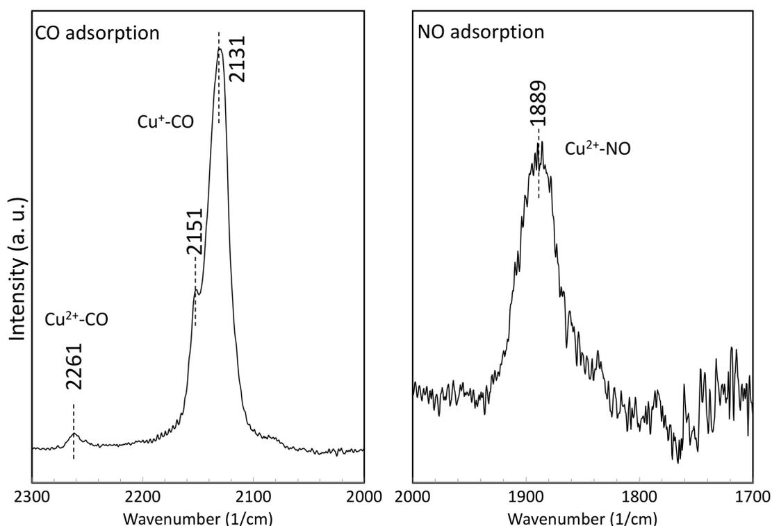
Figure S4: Infrared spectra recorded after CO adsorption (left) and NO adsorption (right) on the Cu-BS sample.
