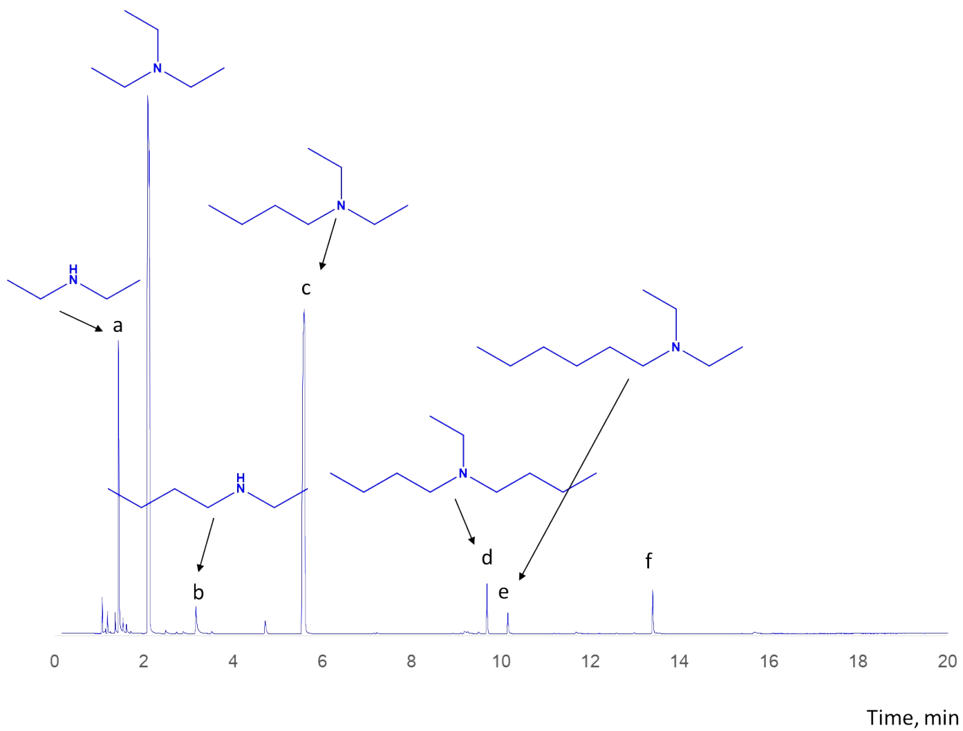
Figure S1. GC-MS analysis after 5h during TEA transformation (2 g TEA, p(N_2)=5 bar, 0.1 g Pd/Al 2 O 3 , 200 °C) with assignment of the products a,b,c,d,e,f in the Figure S2
