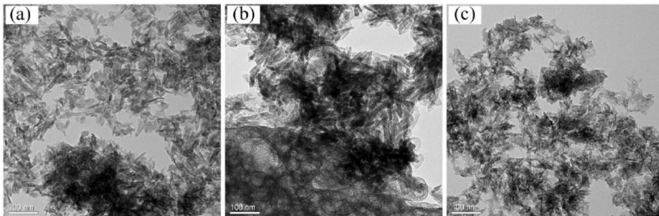
Figure S4. TEM images of Fe-TCP of (a) 2%; (b) 5%; (c) 10%.
