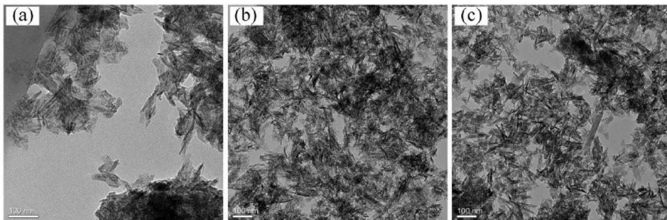
Figure S5. TEM images of Fe-TCP of (a) 2%; (b) 5%; (c) 10%.
