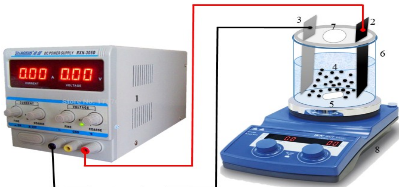
Fig. S2. The batch electrochemical reactor, 1. DC Power supply, 2. Anode electrode ( G/\beta\text{-PbO}_2 ), 3. Cathode electrode (SS316), 4. Simulated 2,4-D solution (including GACs), 5. Magnetic- bar stirrer, 6. Electrochemical cell, 7. Sampling port and 8. Magnetic stirrer controlled
